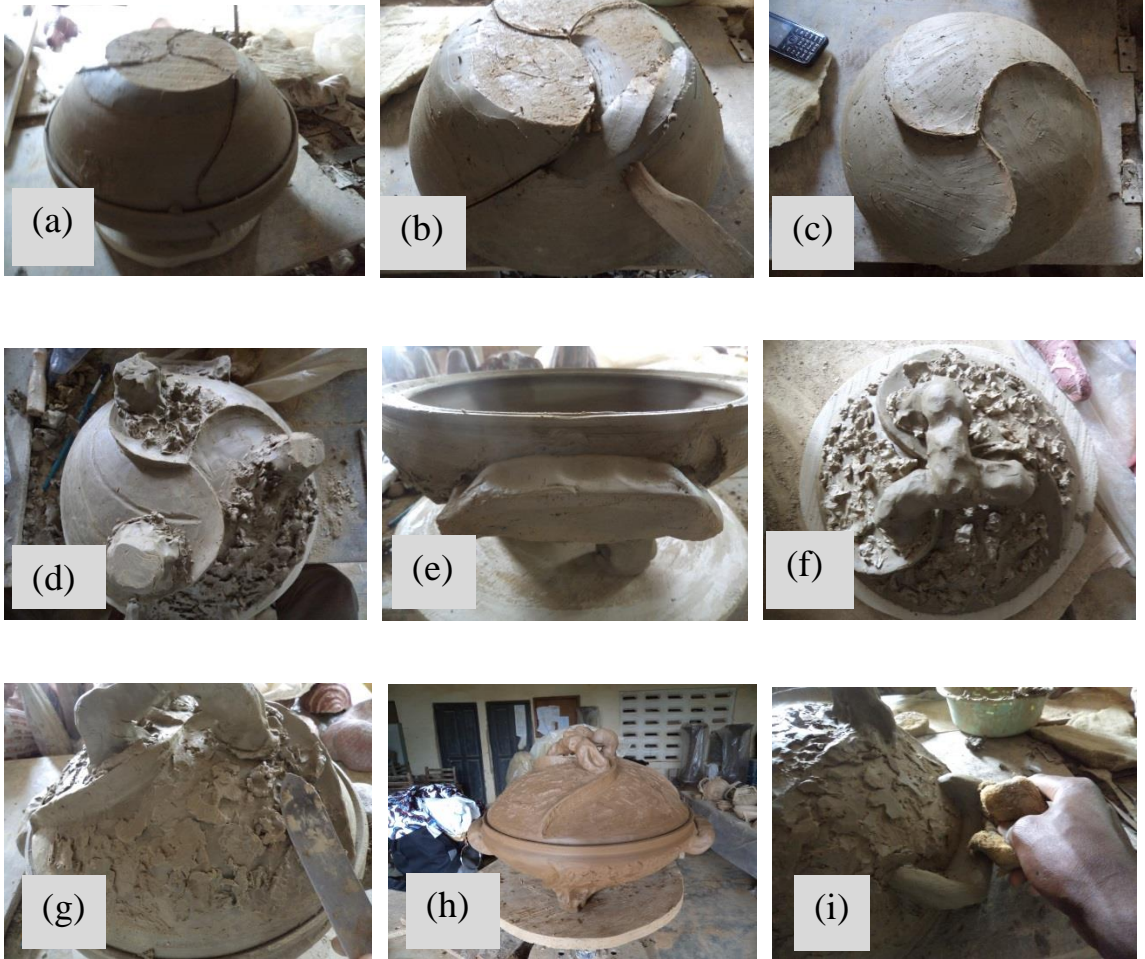
Plate 3- 14: Pictures showing the making of the serving bowls (a) thrown bowl and lid (b) demarcated lines for the foot and handle (c) demarcated lines for foot and handle (d) fixing of foot (e) fixed handles on the bowl (f) fixed handle on the lid (g) decorating with a knife (h) finished bowl with lid (i) cleaning with a foam.
