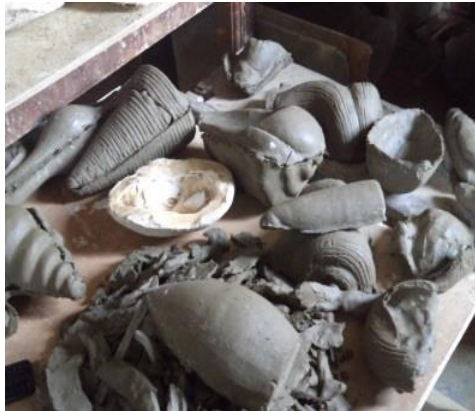
Plate 3- 7: Pressed pieces of seashells removed from the moulds
