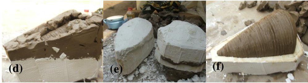
Plate 3- 5: pictures showing the construction of the P.O.P moulds for the seashells (a) Modeled seashell burried halfway in a lump of clay (b) Hard paper used in place of a casting box (c) P.O.P mixture poured on the model (d) The other half of the model yet to be cast (e) Both halves of the model cast in P.O.P and (f) Model burried halfway in P.O.P
