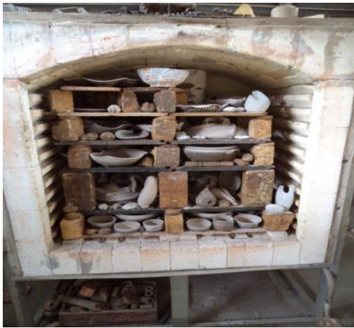
Plate 3- 19: Packed kiln with pottery wares and seashells for gloss firing
