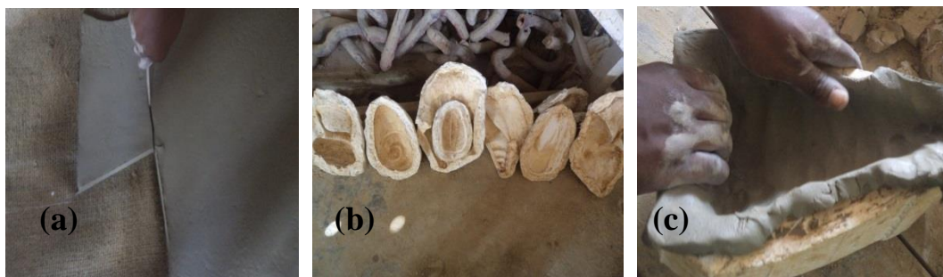
Plate 3- 6: (a) Clay slab (b) P.O.P moulds (c) Pressing clay slab into the mould
