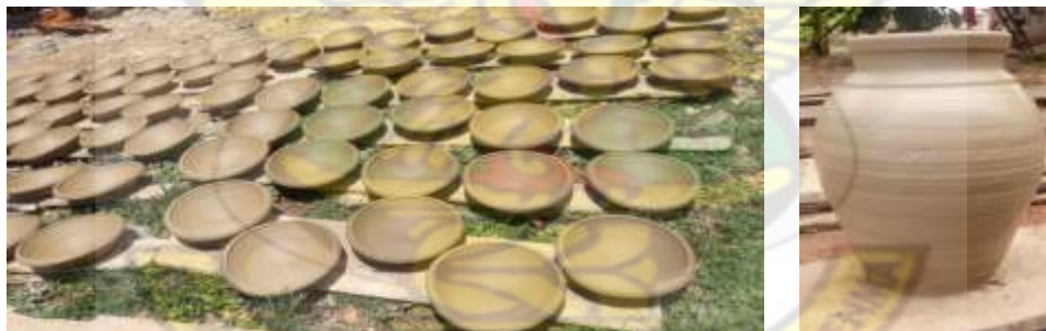
Plate 4.9: Sun-drying method of pottery objects (from the 1960s to date)
