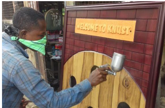
Plate 3.73: Applying lacquer and auto-base clear.
