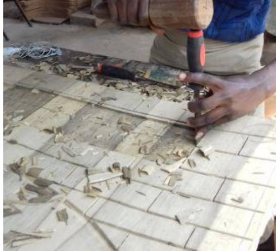
Plate 3.53: carving the space that will hold the plaque
