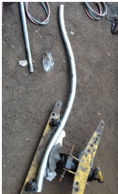
Plate 3.85: The bent pipe ready to be removed
