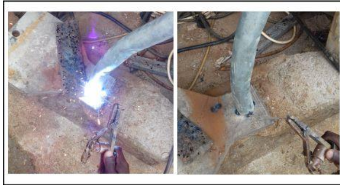
Plate 3.86: Tacking the pipe to the base metal.
