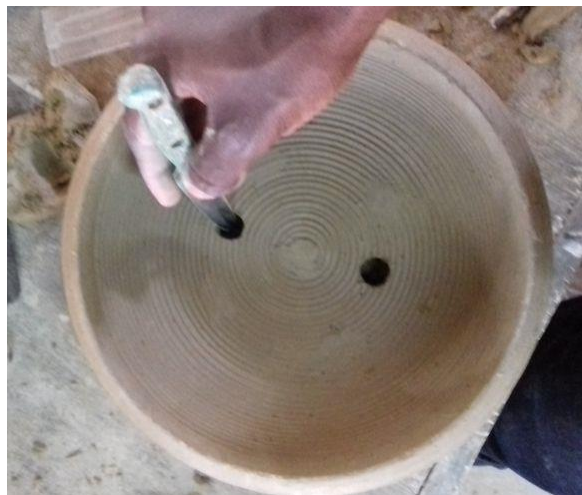
Plate 3.14: creating the two center lockers
