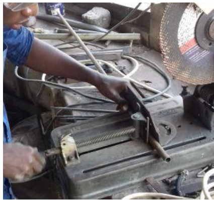
Plate 3.42: marking the length of the tube before cutting
