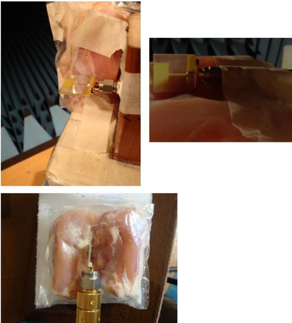
Fig.4.4 Performance of the fabricated flexible pattern reconfigurable antenna on a stuffed animal body.
