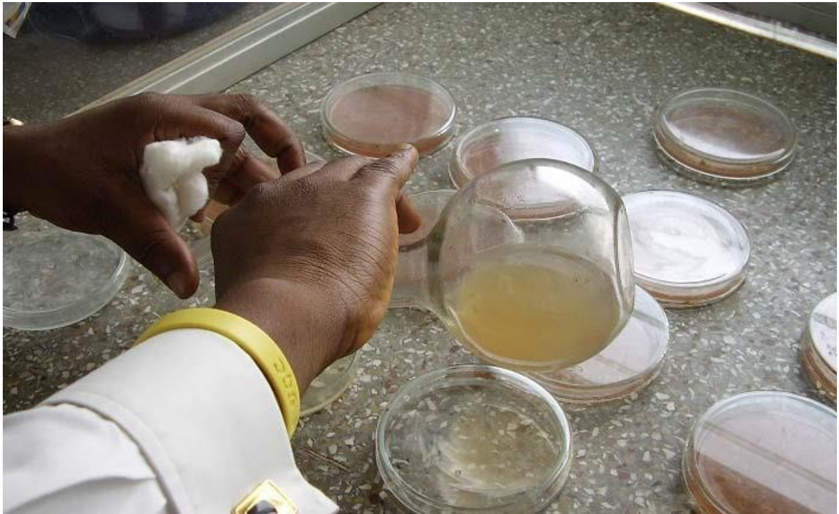
Plate 3. Aseptic pouring of medium into petri dishes.
