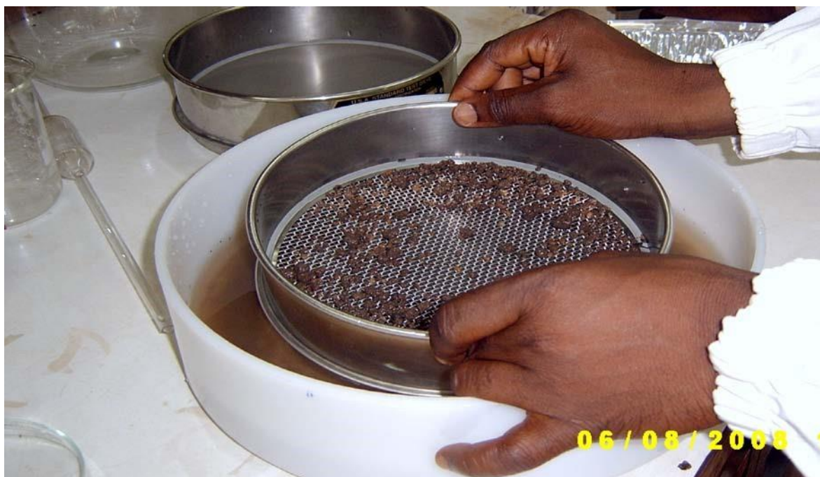
Plate 2. Wet - sieving of whole soil as described by Six et al. (1998).
