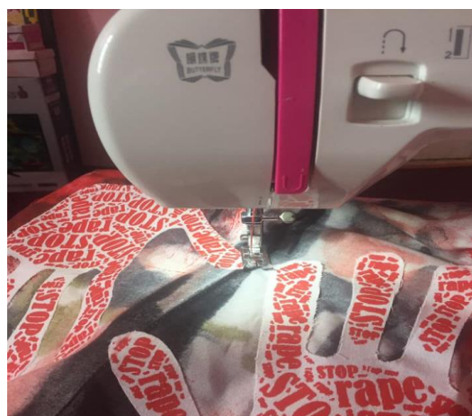
Plate 3.33c: Applique of Image 'Palm' with zig-zag stitches dress after drying out and pressing
