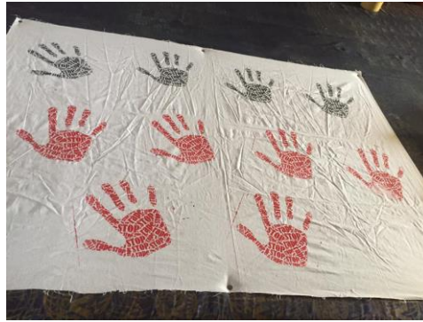
Plate 3.33a: Screen printing of 'Palm' image in Red and Black Print Paste
