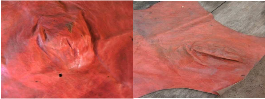
Plate 4.7: Hunch back pocket areas hindering the spread of leather surface.
