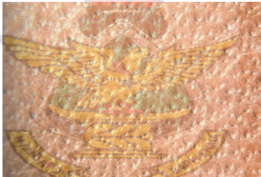
Plate 2.3(b): Hair follicle pattern of calfskin leather (Magnification: x45) (Source: Haines, 1981)
