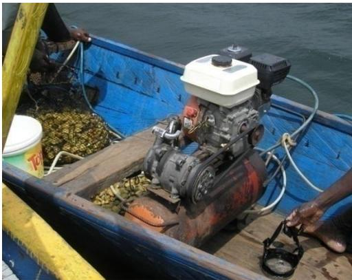
Plate 3.3 *A motorized air compressor*
