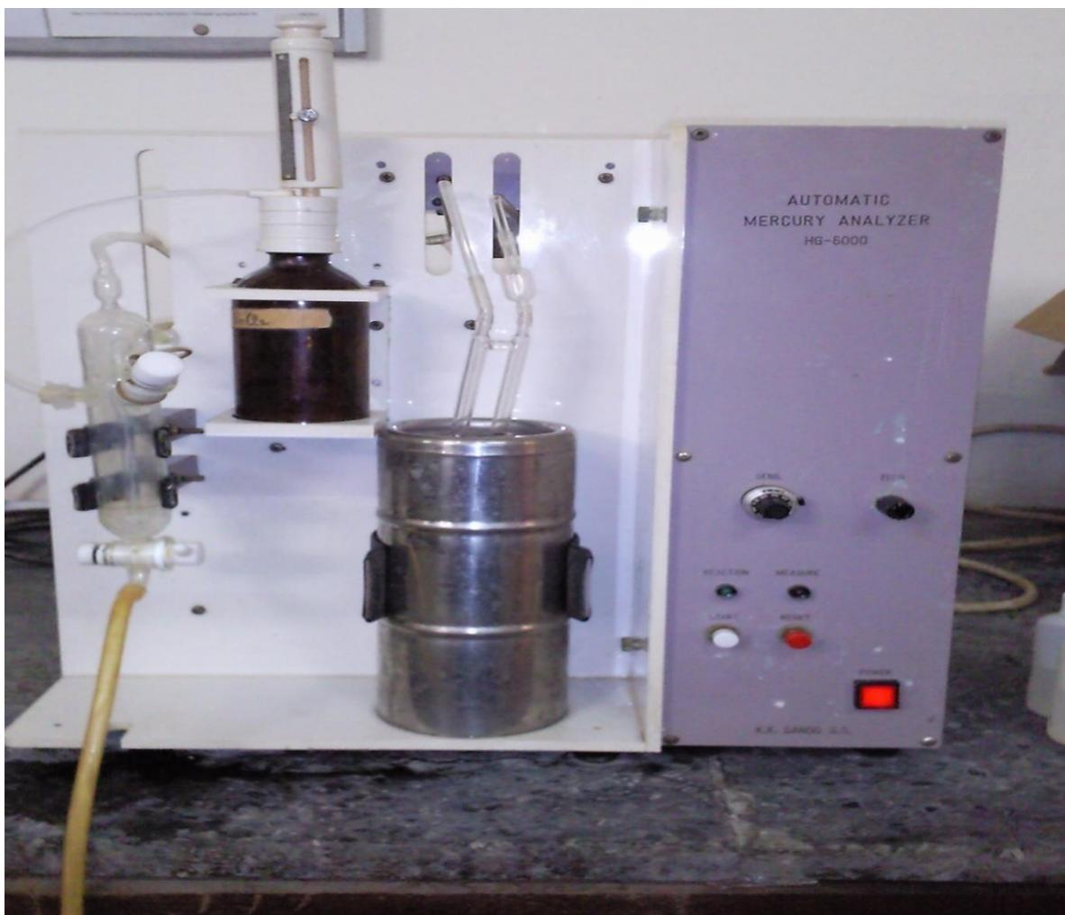
Plate 3.5 *The Automatic Mercury Analyzer (Model HG 6000)*
