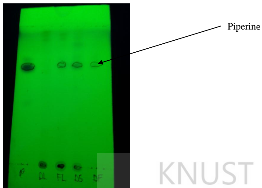
Figure 14: TLC chromatogram of isolated piperine run alongside plant extracts in chloroform: ethylacetate 1: 1 viewed under 254nm UV light
