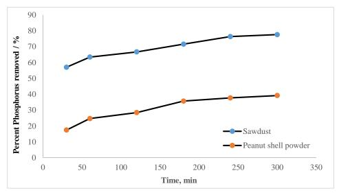
Figure 2. Effect of contact time on phosphorus removal
