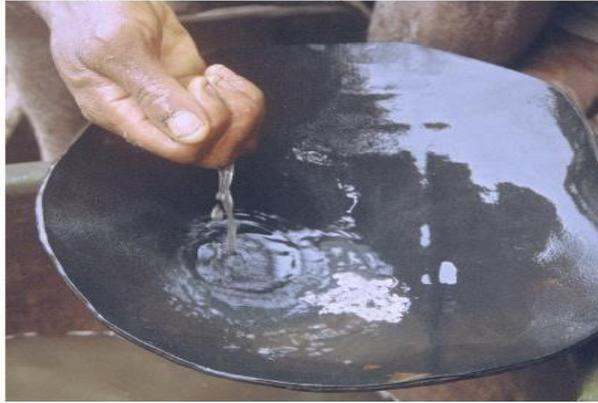
**Figure 1:** Artisanal gold miner washing gold obtained using the gravity method
