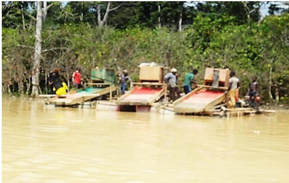
**Figure 8: Felt mats washing of suction gravel, mud, and rocks in Pond at Yale.**
