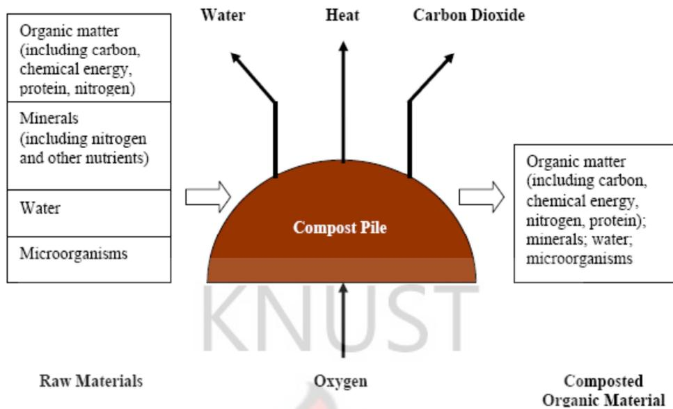
**Figure 2.1: Composting process schematic diagram (from NRAES, 1992)**
