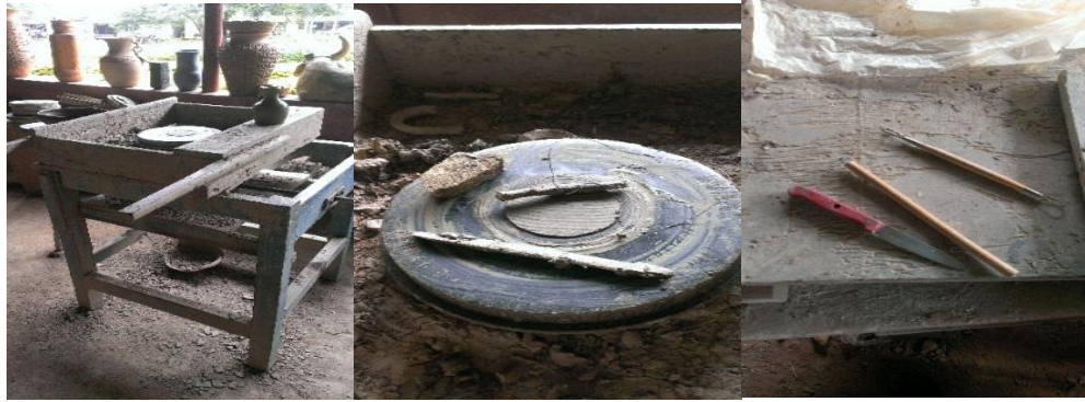
Plate 27. Tools and materials for throwing
