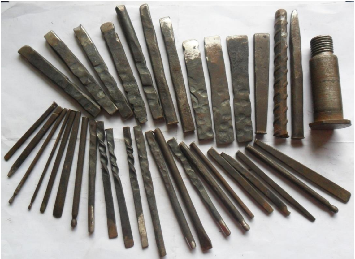
Figure 27: (2013) Repoussage tools with varied working ends
