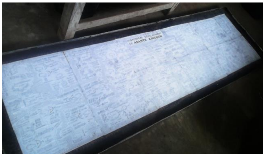
Figure 42: (2013) Copper sheet with pasted working drawing
