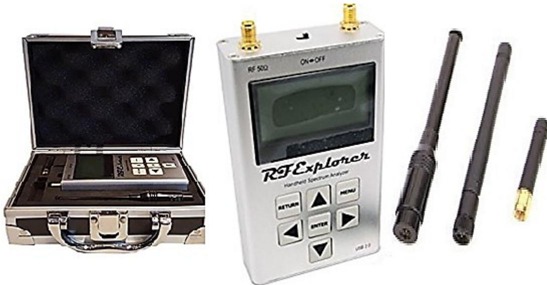
**Figure 3.6 RF Spectrum Analyzer with Antennas**
