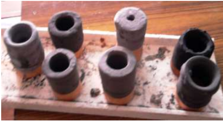
Figure 3.1 Prepared glazed test pieces ready for firing
