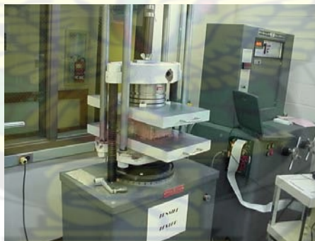
Figure 2.9 compression test set up – Tinius Olsen universal testing machine
