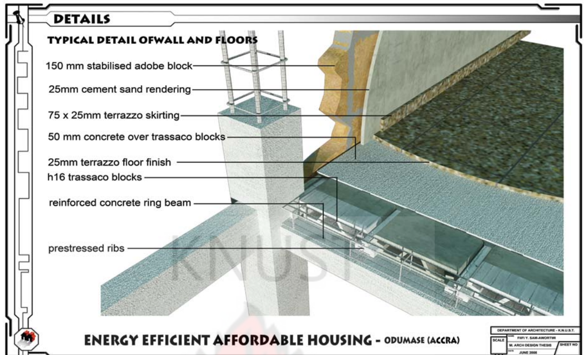
Figure 5.40 Typical detail of floors and walls
