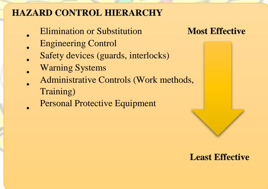
**Figure 3.1: Hazard Control Hierarchy**
