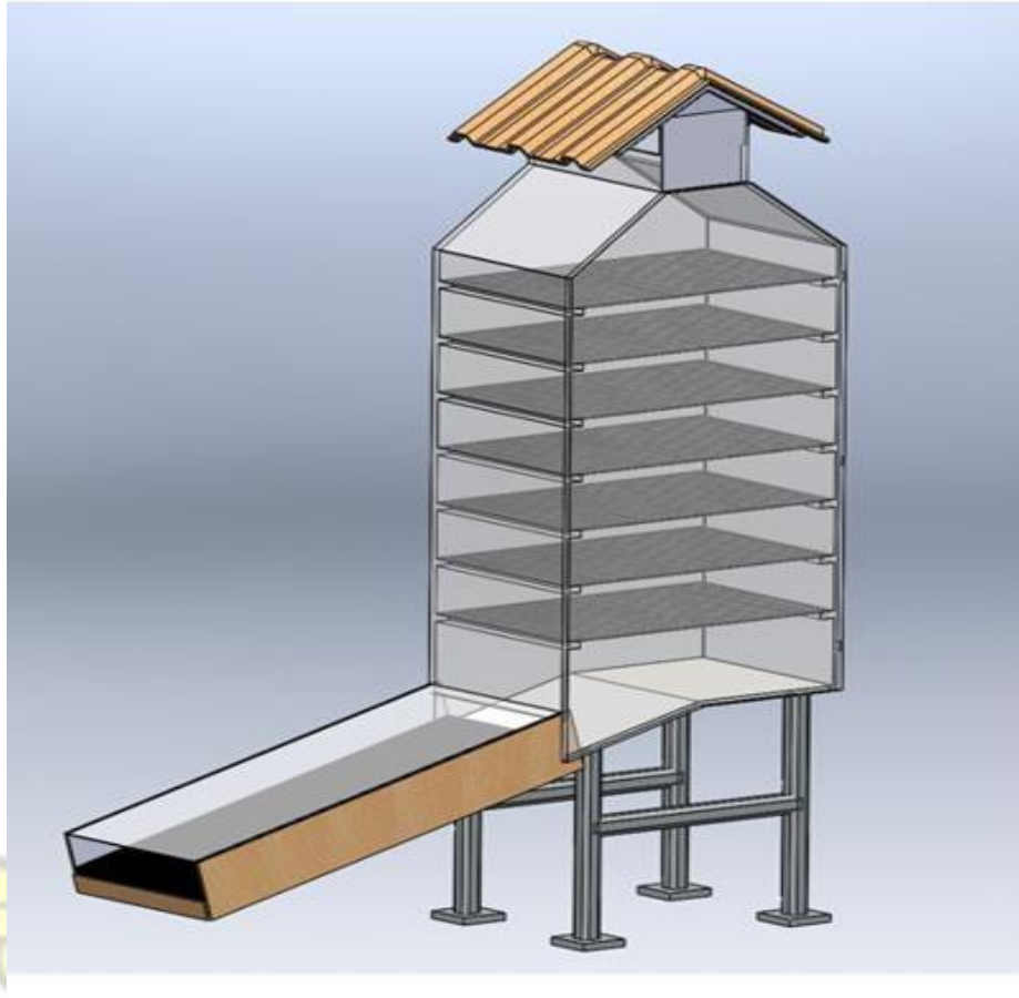
Figure 3. 1: A 3D AutoCAD drawing of proposed Dryer
