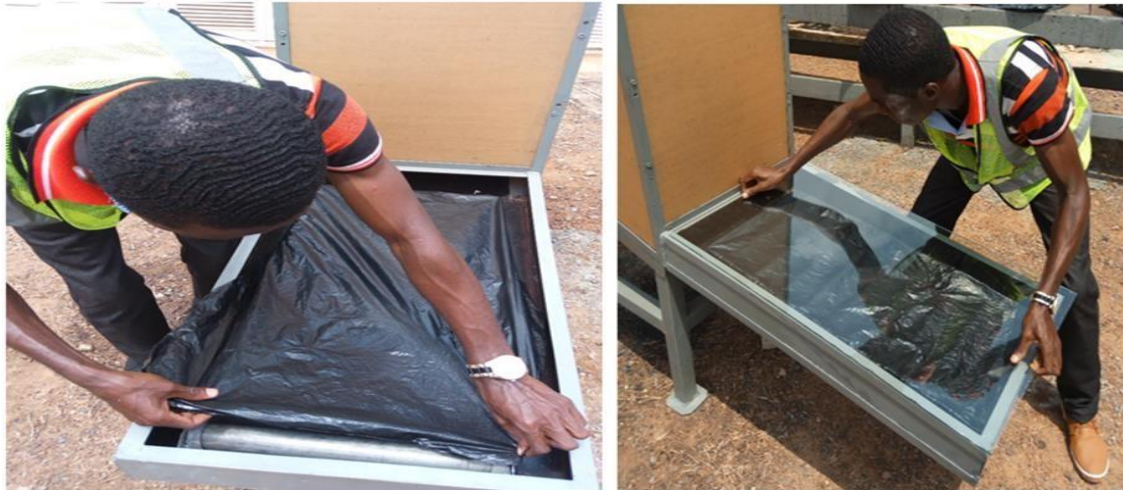
Figure 3. 8 Pictorial view of a black polythene used to cover the surface of the aluminium pipes and inserted into the crop dryer coved with glass
