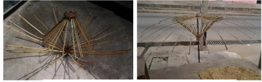
Plate 5.5d and 5e: Completed framework of the umbrella Source: studio work (2015)
