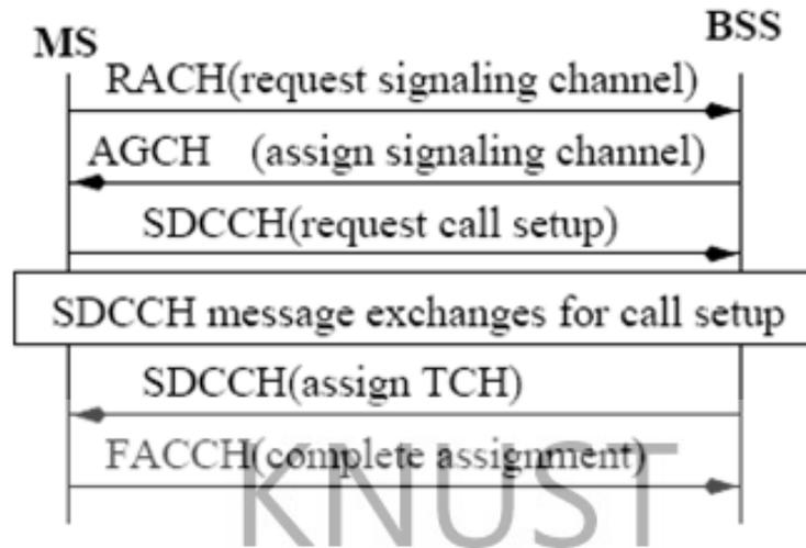
Figure 2.3: GSM Call Origination (Radio Aspect) [9]
