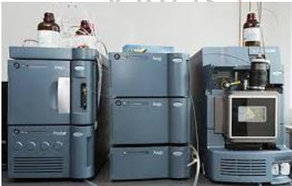
Figure 3.5 Pictorial representation of Waters SQD2 quadrupole mass spectrometer
