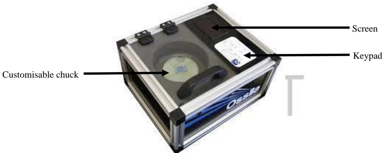
Figure 3.7 Pictorial representation of a spin coater with part labelled
