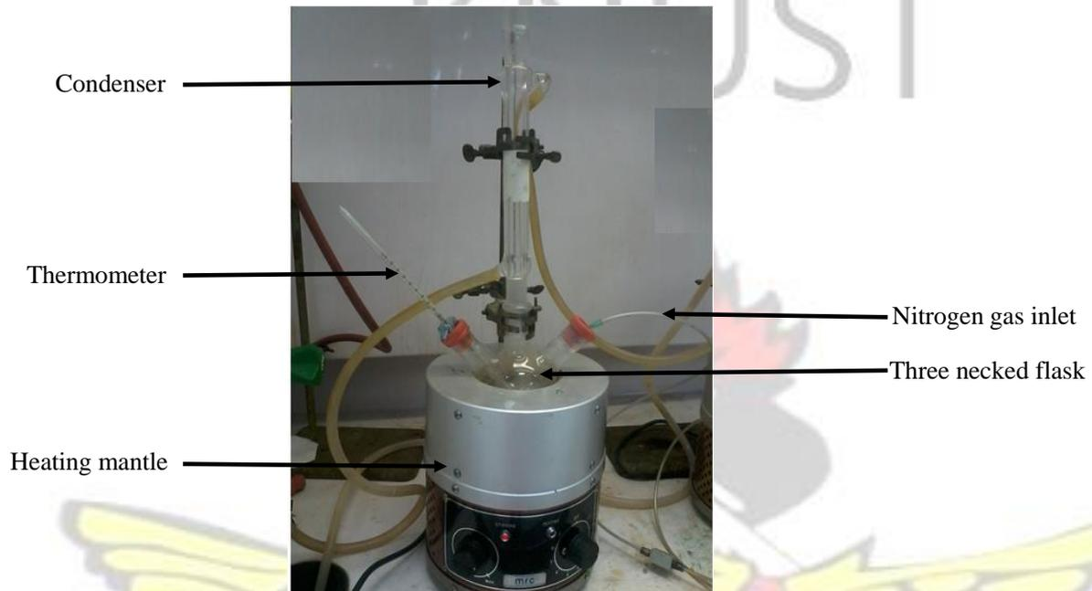
Figure 3.8 Pictorial representation of hot injection set up
