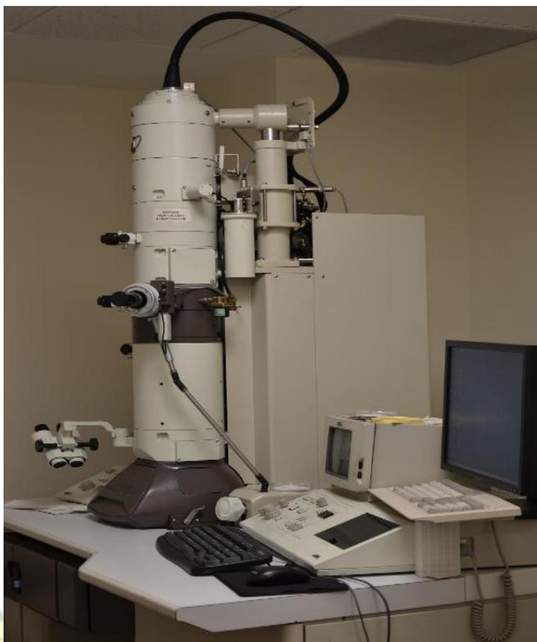
Figure 3.11 A photograph of JEOL 1010 Transmission electron microscope
