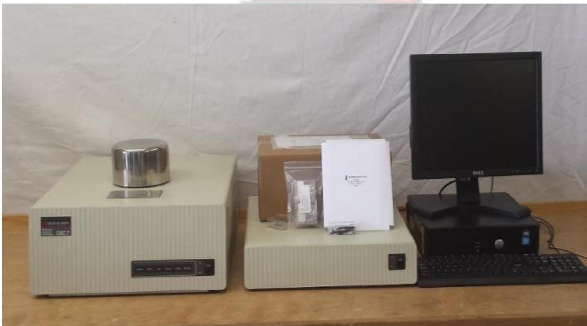
Figure 3.6 Pictorial representation of Perkin-Elmer TGA7
