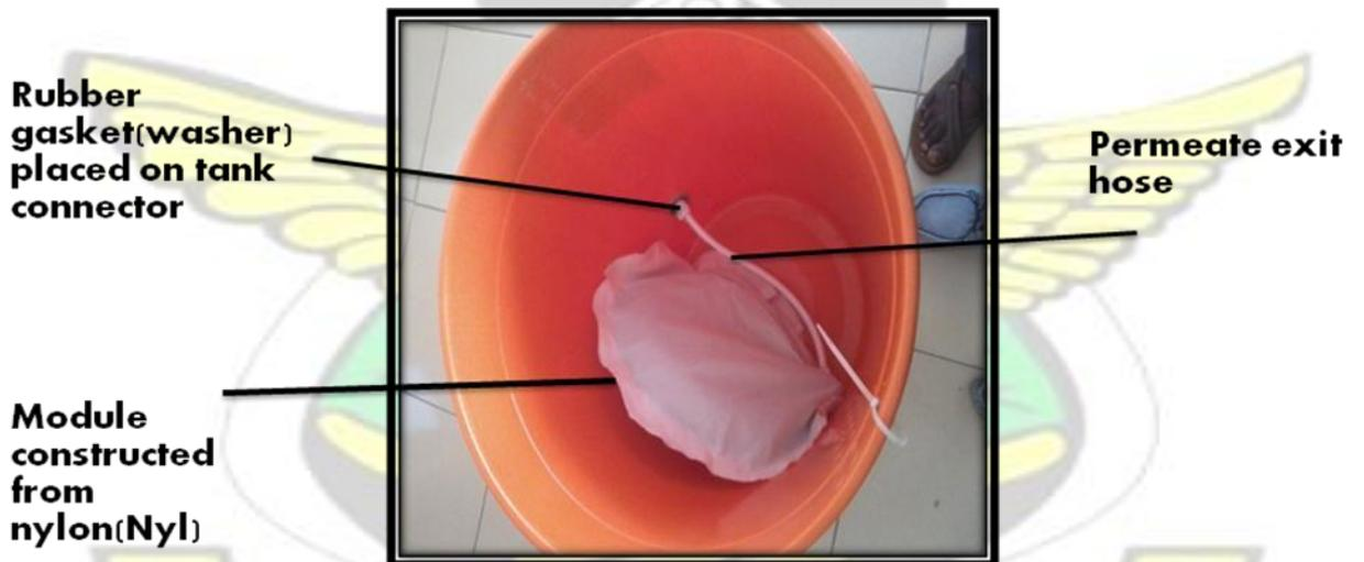
Rubber gasket(washer) placed on tank connector
