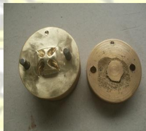
Fig. 82: Drilled dots on a Die and its corresponding punch
