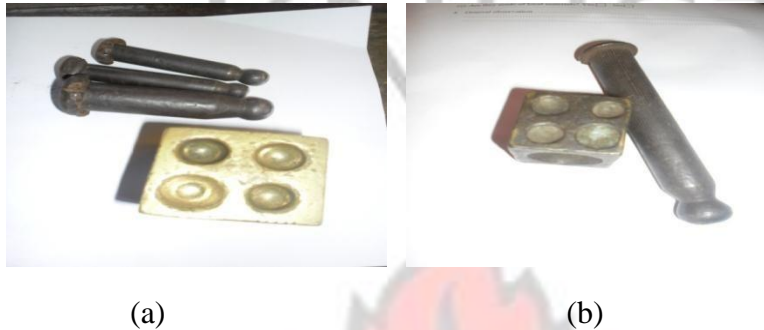
Fig. 3a & 3b: Samples of doming blocks and metal Punches used by the goldsmiths
