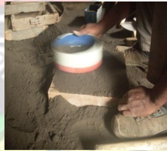
Fig. 50: Sieving of sand on mould surface
