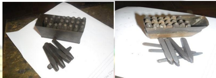
(a) (b) Fig. 4a & 4b: Letter Punches used by the Goldsmiths
