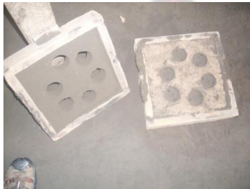
Fig. 56: Prepared sand moulds
