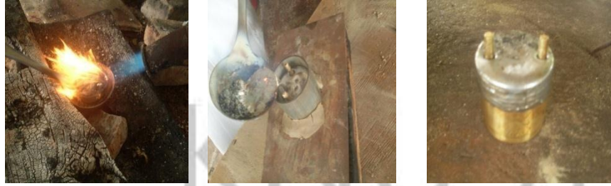
a: lead melting b: casting lead c: cast lead pattern Fig. 63a, b & c:
