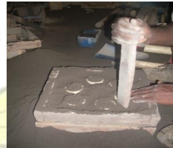
Fig. 53: Application of parting sand. Fig. 54: Ramming of the cope with sand.
