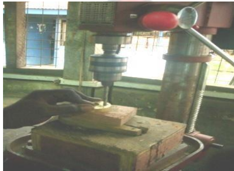
Fig. 78: Drilling the holes through a die
