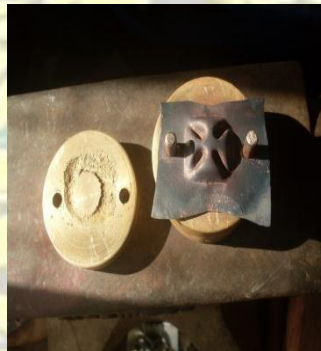
Fig. 89: 2 nd Embossing after annealing
