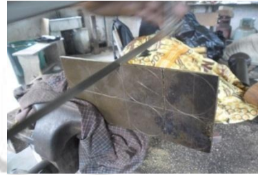
Fig. 26: Cutting of brass figure into squares
