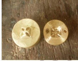
Fig. 75: Die and Punch used for Testing
