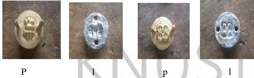
Fig. 65: Other punches and their lead dies
