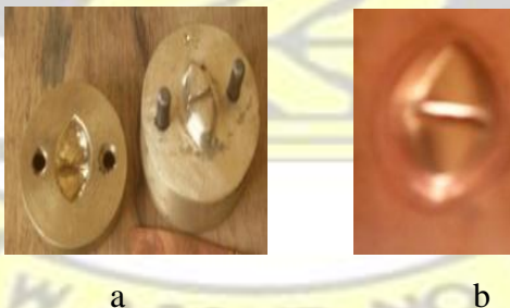
Fig.106a & b: Perper Die/punch set and embossed piece
