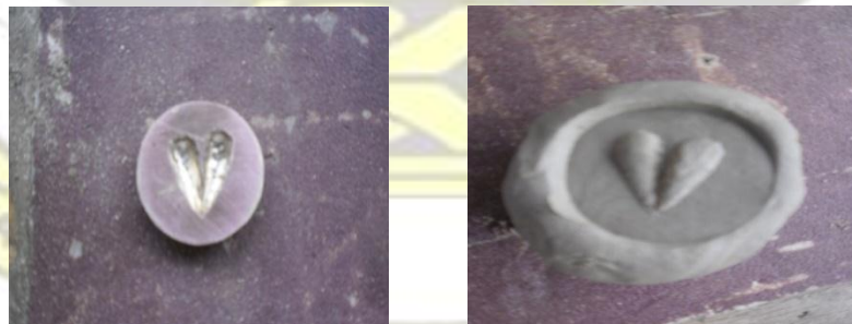
Fig. 22: Sunk image as die model. Fig. 23: High relief impression
