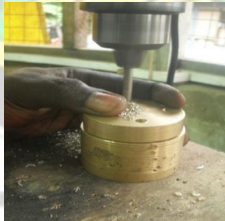
Fig. 79: Drilling holes through a die and a punch
