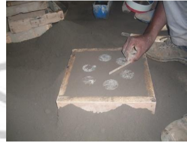
Fig. 51: Pressing and ramming processes. Fig. 52: The finishing of the first mould
