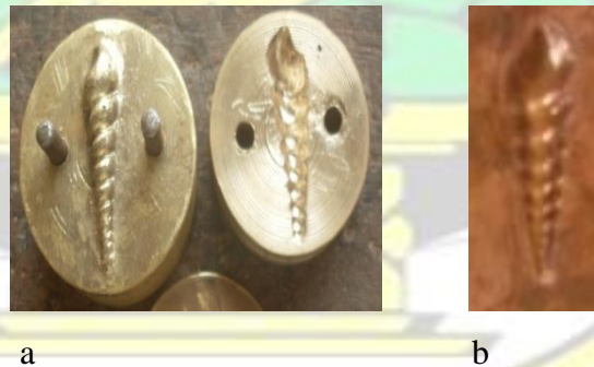
Fig. 103a & b: Ahoɔfɛ ntua ka Die/punch set and embossed piece
