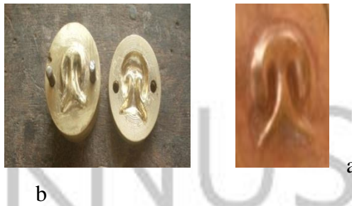
Fig. 101a & b: Papaye Die/punch set and embossed piece
