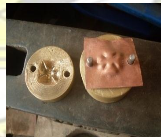
Fig. 87: 1 st Embossing process
