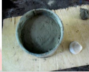
Fig. 33: Casting flask and prickly cockle shell
