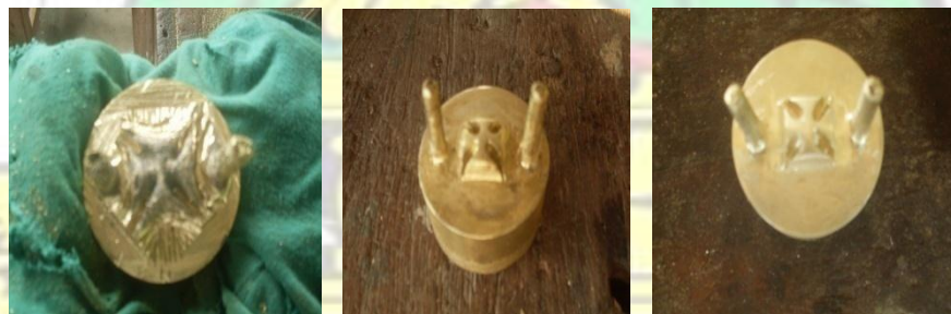
Fig. 61: Stages in finishing the punch
