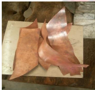
Fig. 84: Milled copper sheets
