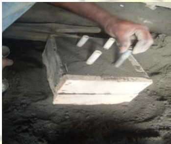
Fig. 69: Pipes on lead dies
