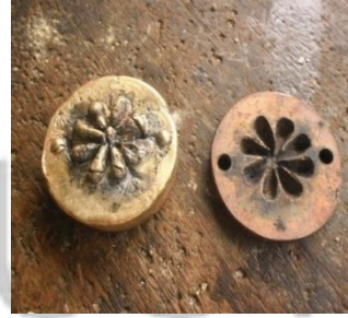
Fig. 41: Cast brass and die
