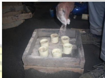
Fig. 53: Application of parting sand. Fig. 54: Ramming of the cope with sand.
