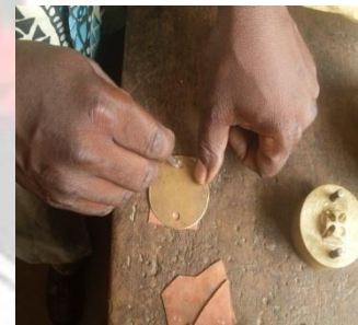
Fig. 85: Marking for drilling
