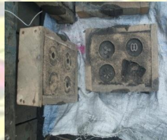
Fig. 70: Prepared sand moulds
