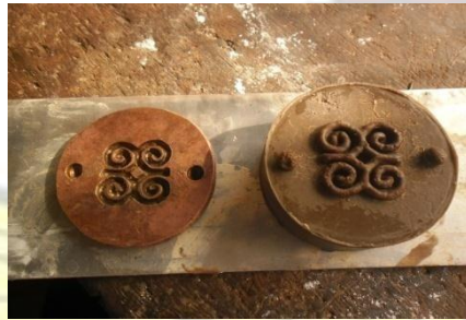
Fig.36: Die and pattern cast in wax and POP mixture
