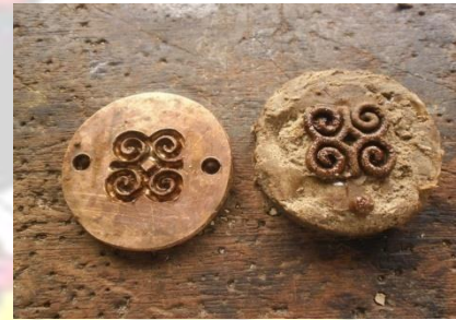
Fig.37: Die and pattern cast in wax, POP and clay
