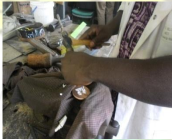
Fig. 30: Sinking of the dies models
