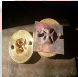
Fig. 81: Embossed Element with pilot pins
