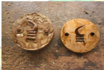
Fig. 38: Die and cast pattern in wax, clay and POP
