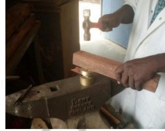
Fig. 76: Testing Embossing Process
