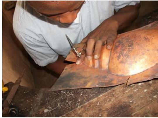
Plate 3.51 – Piercing off excess metal
