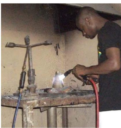
Plate 3.30 – Soldering the cone
