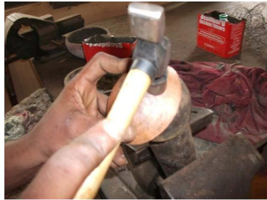
plate 3.10 – raising the disc on a metallic stake.
