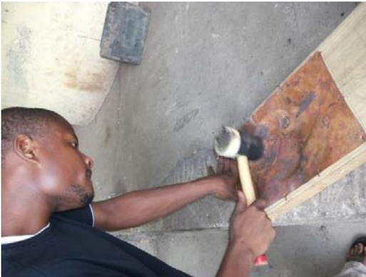
Plate 3.44 – Pushing with a rubber mallet
