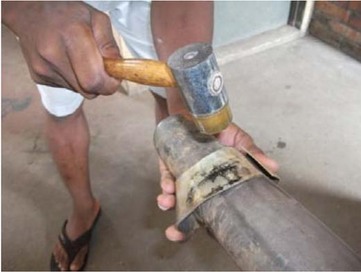
Plate 3.60 – Forming the cone on a stake
