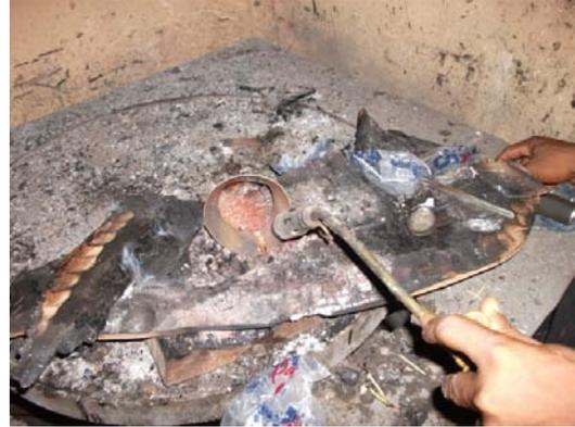
Plate 3.61 – Soldering the joint
