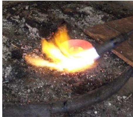
plate3.17 - soldering the assembly onto the brass base
