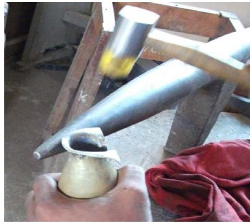
Plate 3.37 – Raising the work on a stake
