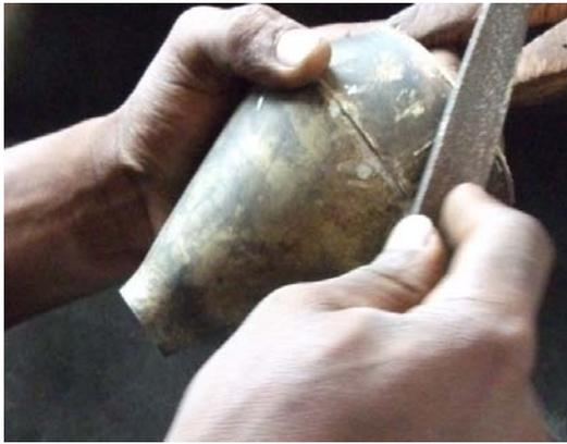
Plate 3.64 – Filing off excess metal
