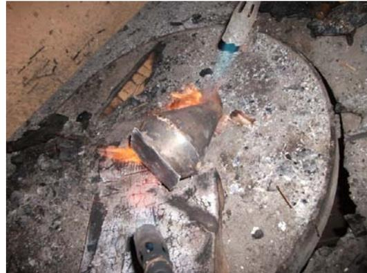
Plate 3.63 – Soldering the two parts together
