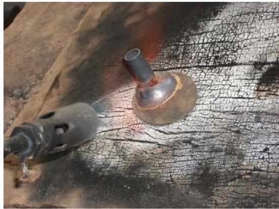
plate 3.20- soldering the tube, dome and the oval plate
