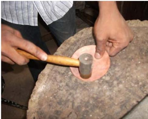
Plate 3.9 – sinking the disc on a block of wood.
