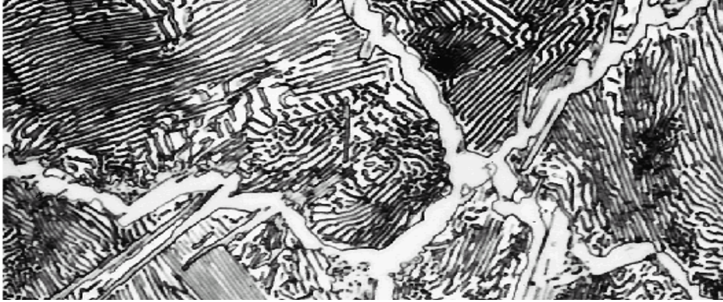
Fig.2.8 Microstructure of hypereutectoid steel [44]
