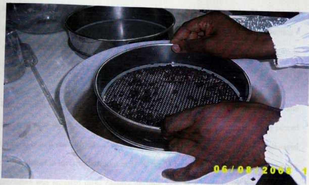
Plate 2. Wet - sieving of whole soil as described by Six et al. (1998).
