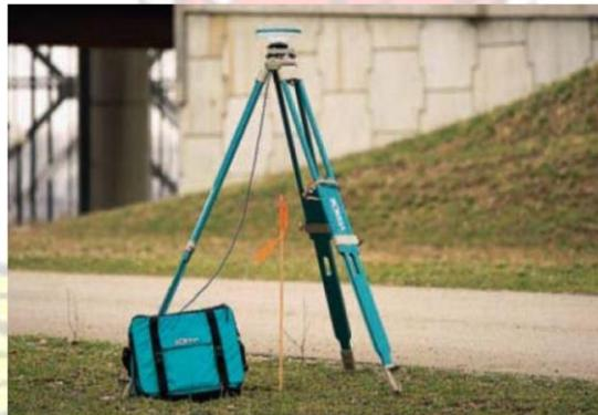
Figure 3. 4 A SOK702 antenna mounted on a tripod for data collection
