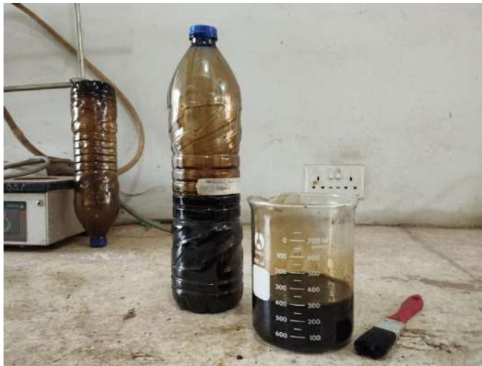
Figure 154 | The CNSL, ready for coating the wood. At the KNUST Department of Wood Science and Technology. Photo credit: Rebecca De Marchi
