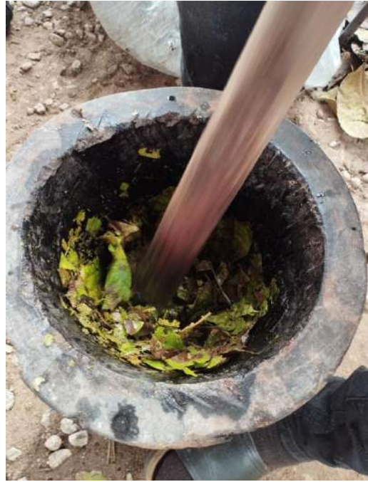
Figure 147 | Cashew green leaves pounded for the tanning process. At the KNUST Leather Section. Photo credit: Rebecca De Marchi
