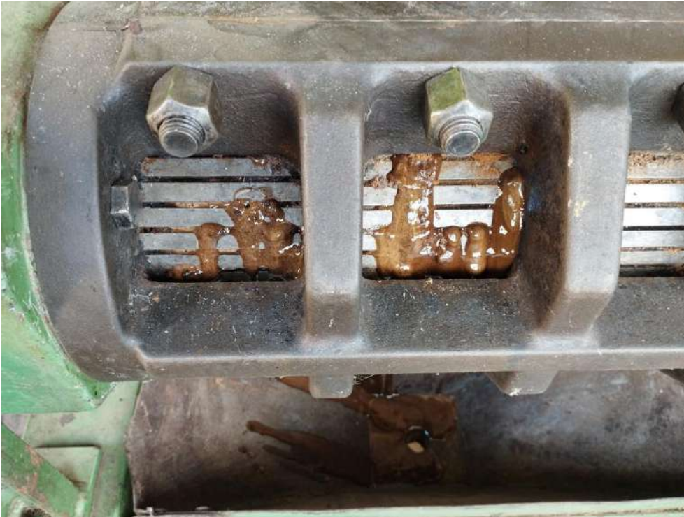
Figure 151 | Extraction of the cashew nut shell liquid CNSL. At the KNUST Laboratory of the Agricultural Faculty. Photo credit: Rebecca De Marchi
