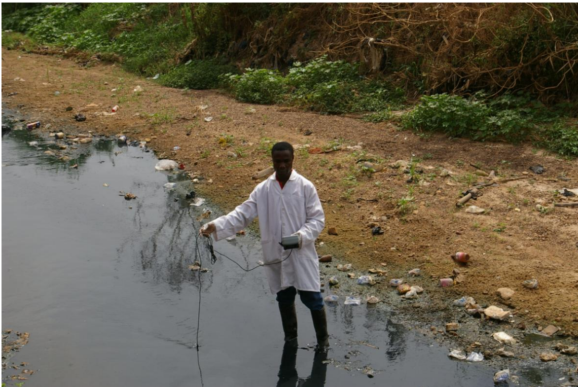
Plate 8.6.7: Taking the DO, pH, and Temperature at Atonsu sampling location.
