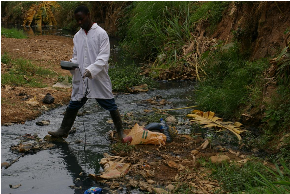
Plate 8.6.5: Taking the DO, pH, and Temperature at Moshie Zongo sampling location.
