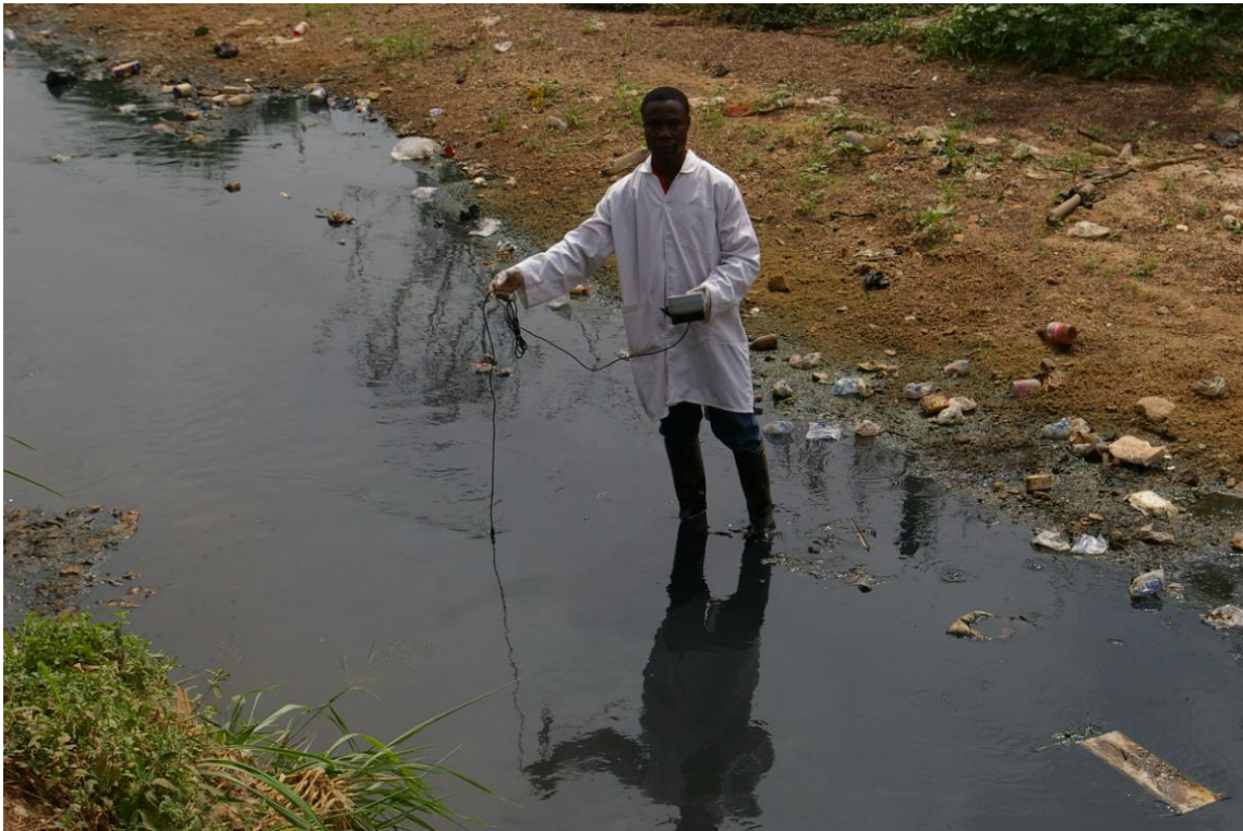
Plate 8.6.7: Taking the DO, pH, and Temperature at Aboabo sampling location.
