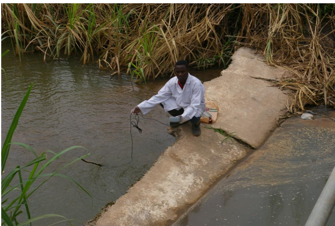
Plate 8.6.4: Taking the DO, pH, and Temperature at Duase sampling location.
