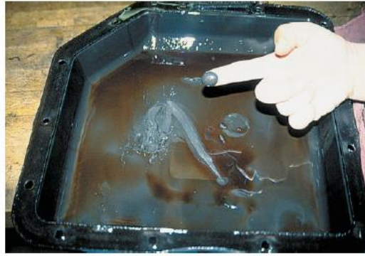
Figure 2.19 Wear material in the bottom of an automatic transmission pan,
