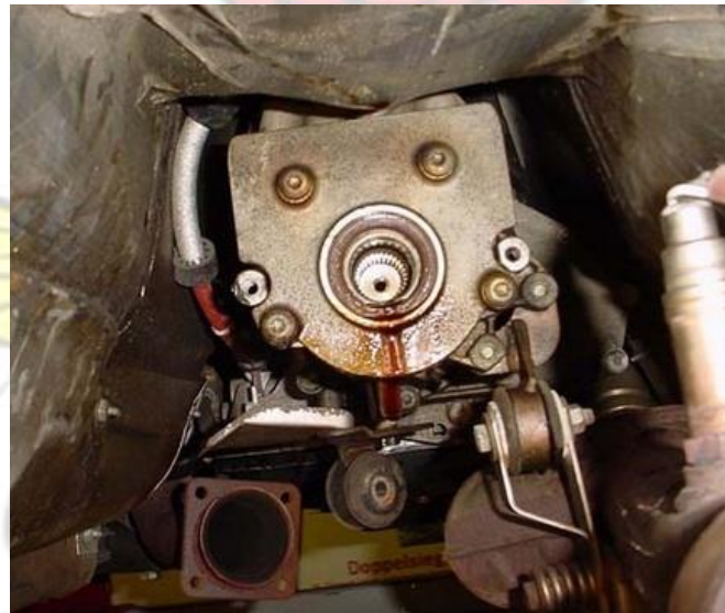
Figure 2.23 Transmission output shaft seal after removing output flange
