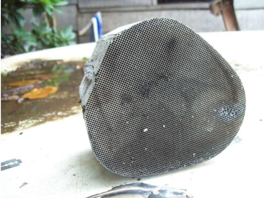
Figure 2.4: A pictorial diagram of a used ceramic honeycomb.
