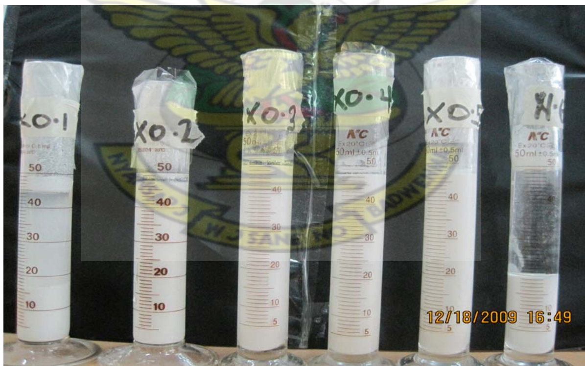
Fig. 3.5.5 Sedimentation volume of xanthan gum suspension after redispersion
