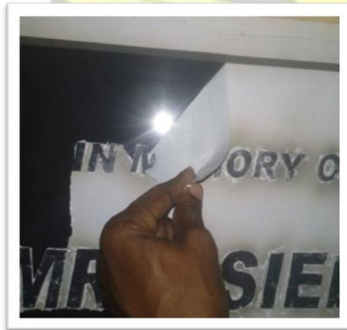
Plate 31: Removing the stenciled sticker Plate 32: Pieced aluminium text firmly adhered Step 4: the finished work was then washed to remove dirt and excess sealant.
