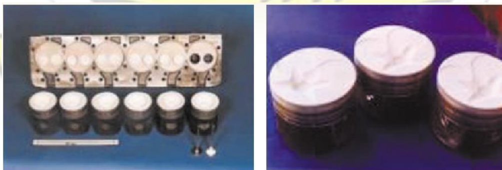
Figure 2.17: Ceramic components in automotive engines Source: Dr.-Ing. Dipl.-Ing. (2004)
