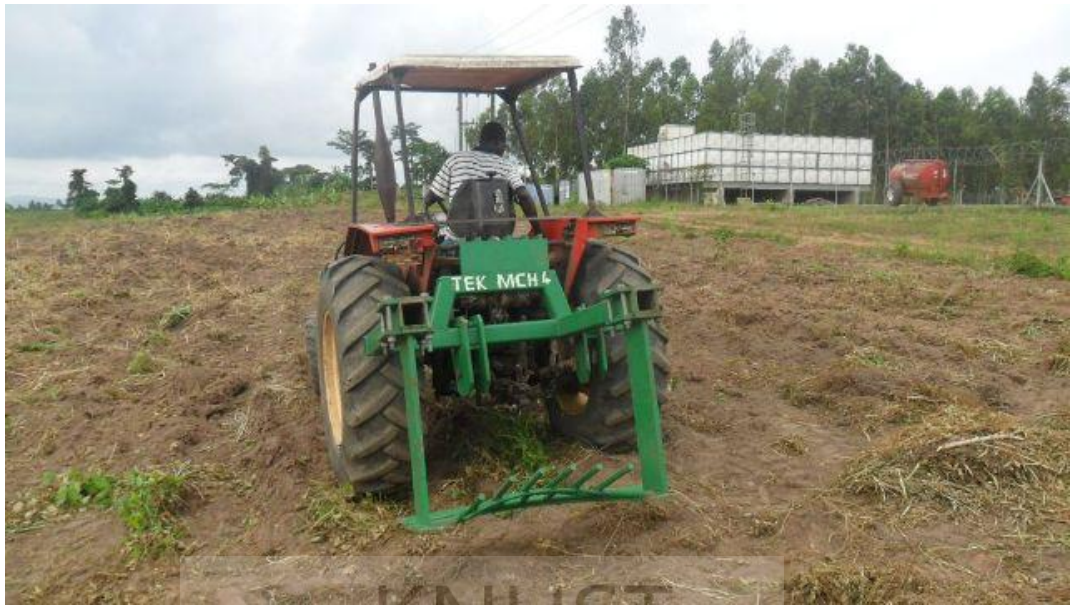
Figure vii: TEK MCH 4 hitched to a tractor in transport position
