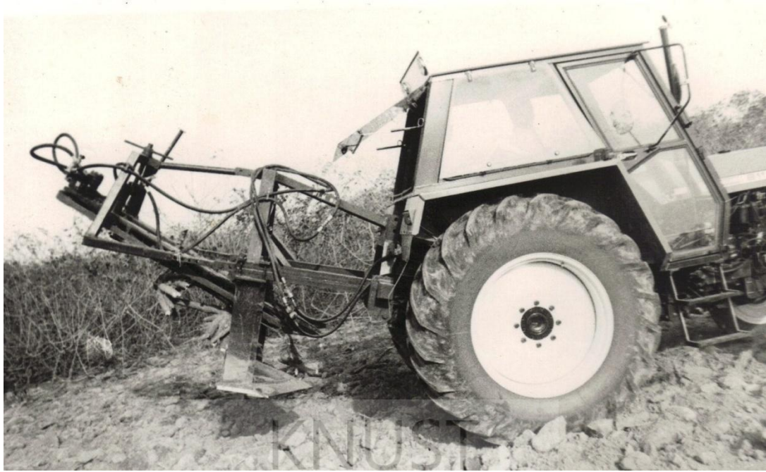
Figure 8: Leipzig Mechanical Cassava Harvester Prototype in operation (Source: Bobobee et al., 1994)
