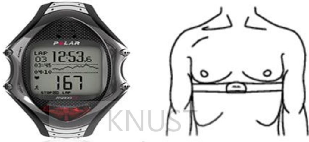
Figure 24: The Polar (RS 800 CX) watch and chest strap as worn by a person
