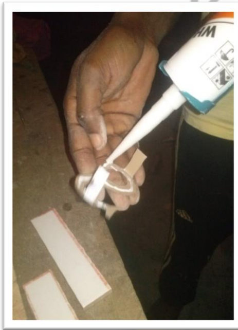
Plate 19: Applying silicone to back of font
