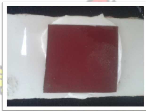
Plate 3: Surface adhesion test of metal and ceramics using silicone sealant
