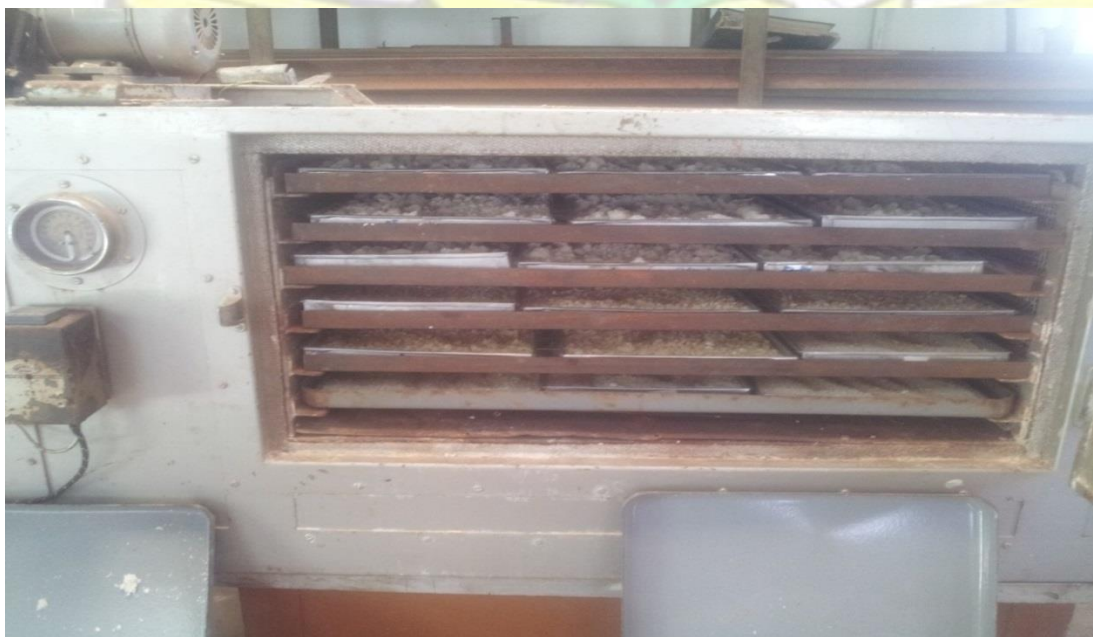
Figure 3. 2 Mechanically ventilated hot air dryer with cassava samples for drying
