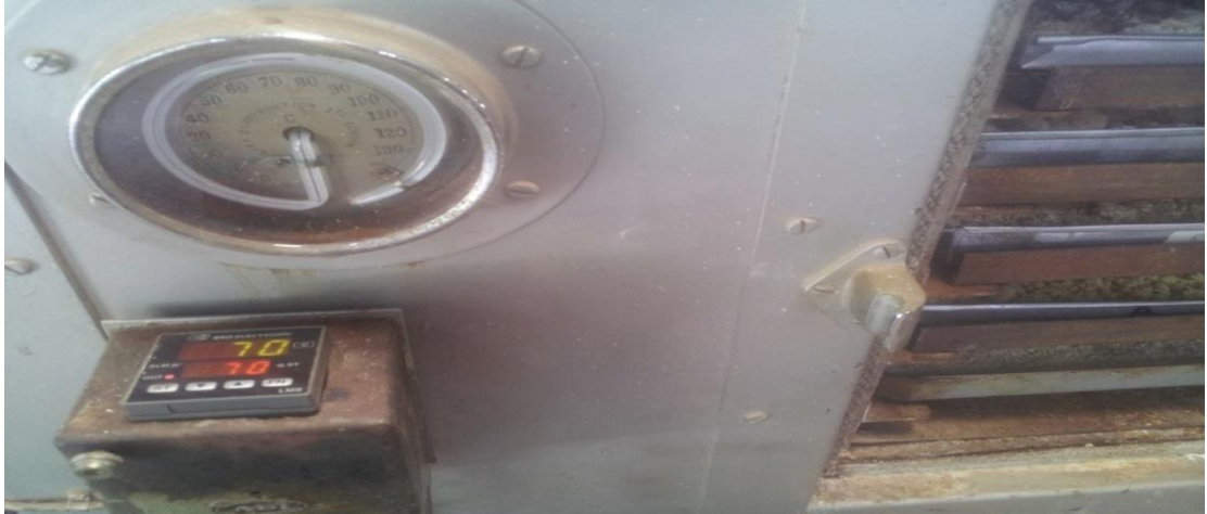
Figure 3. 3 Mechanically ventilated hot air dryer showing the temperature display unit
