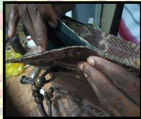
Plate 4.53 (b): Fixing of gusset
