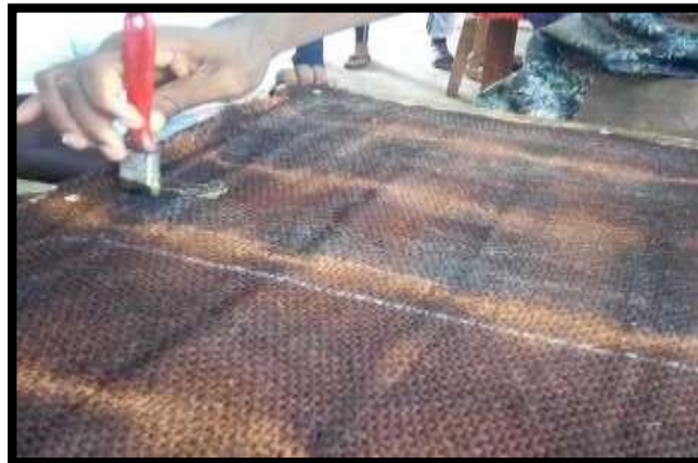
Plate 4.42: Glue application on jute prior to paper attachment.
