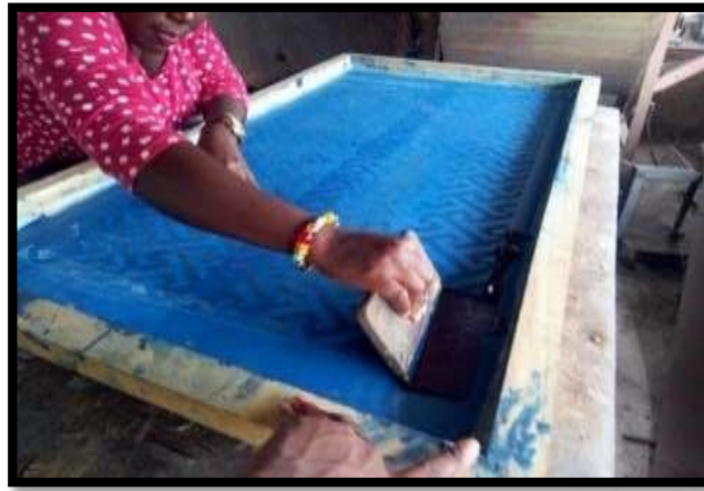
Plate 4.13: Screen printing on the jute using acrylic and printing paste.
