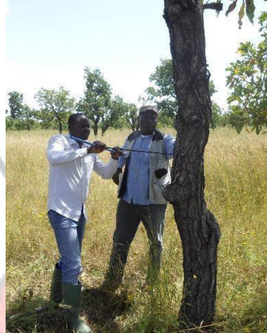
Picture 3. 2 Techniques of extraction of measurement in the wood sample using increment borer. (CHABI, 2014)
