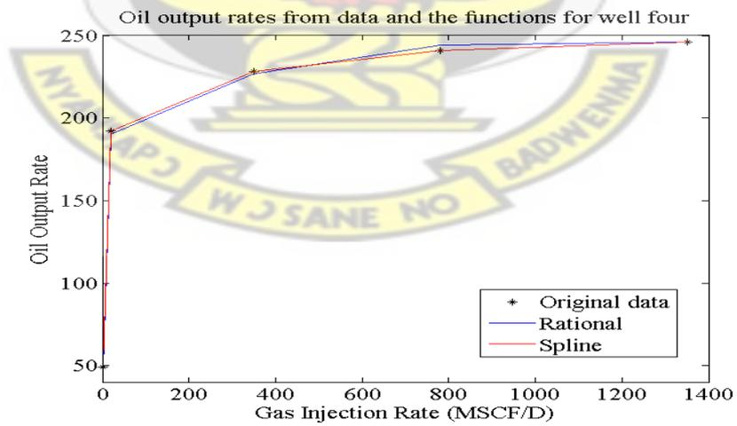
Figure 4.4: Plot of Oil Output versus Gas Injection for Well Four.
