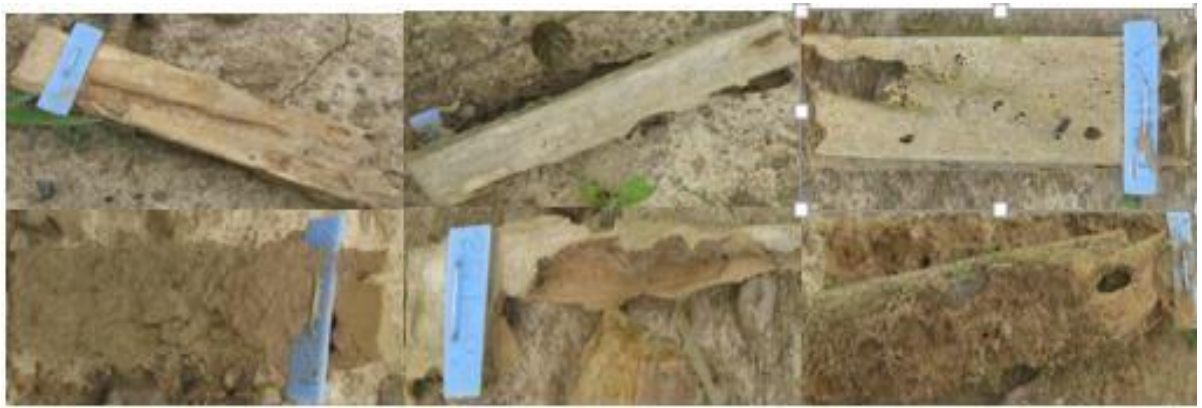
Plate 5.3: Failed heartwood stakes of A. robusta stem by the 16 th week of exposure
