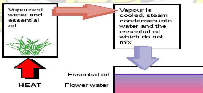
Figure 2.2 Flow process of steam distillation method
