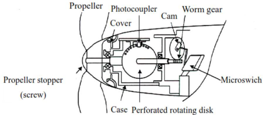
**Figure 2.13: Optical Pulse Generator-Type of Propeller Anemometer**
