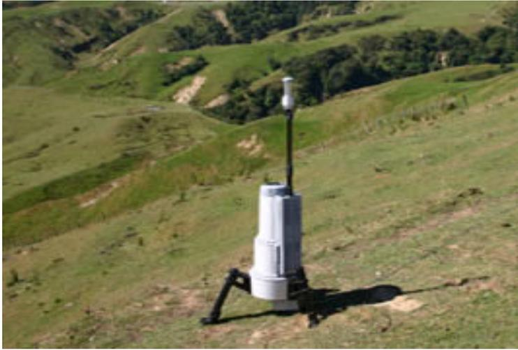
**Figure 2.18: ZephIR Laser Anemometer.**
