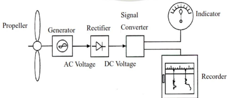
**Figure 2.12: Signal Flow Diagram**
