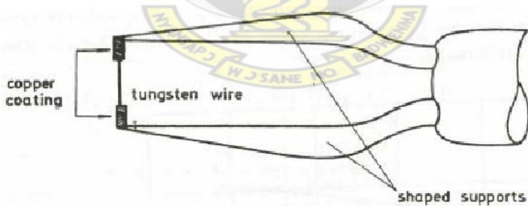
**Figure 2.16: Typical Hot-wire Probe Geometry**
