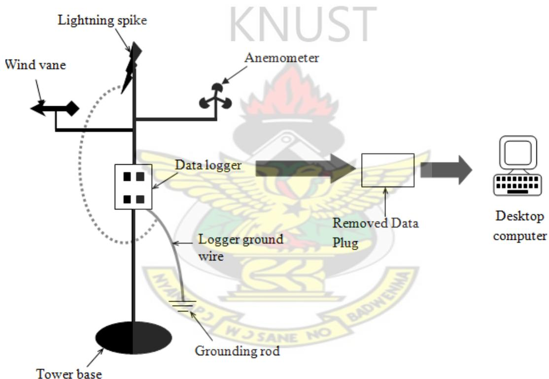
**Figure 3.1: Layout of Experimental Set-Up**
