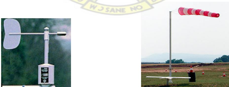
**Figure 2.5: Vector 200P Wind Vane and a Wind Sock**
