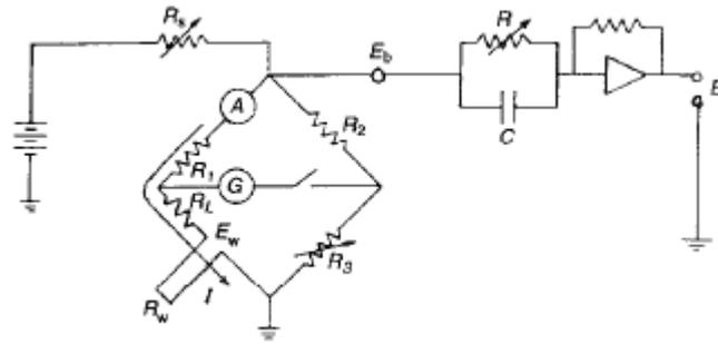
**Figure 2.14: Constant Current Anemometer Bridge Circuit**
