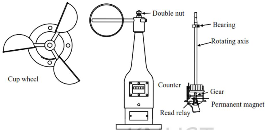
**Figure 2.8: Three-Cup-Wheel Wind-Path Anemometer**
