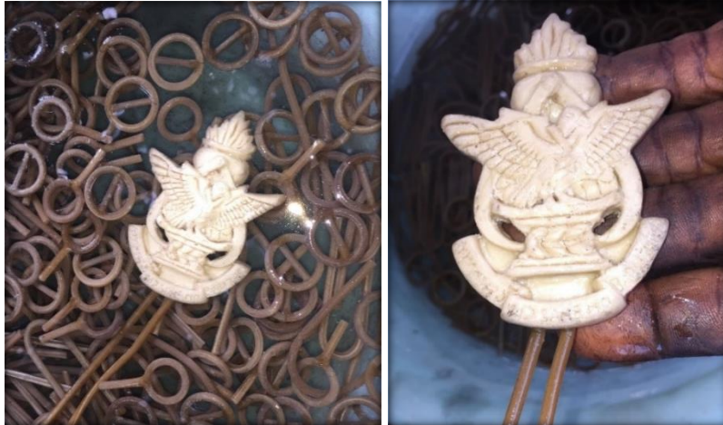
Plate 3.61: Shows soaking of the model in water Plate 3.62: Shows fixing of runners.
