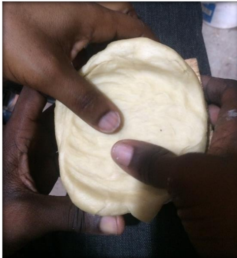
Plate 3.49: Shows plastic bee wax being pressed in the POP mould to pick the emblem.
