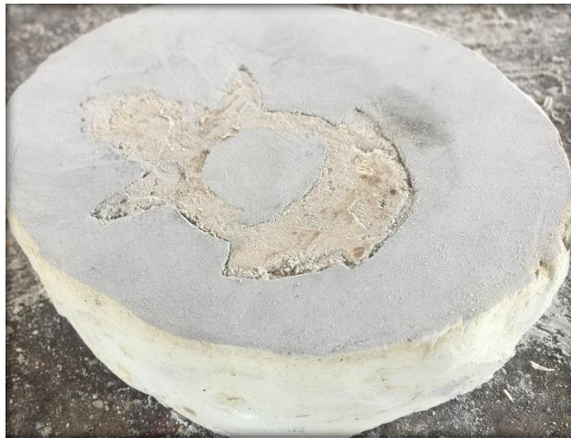
Plate 3.59: Dried cement turned upside down, thus wax is seen stuck in the middle
