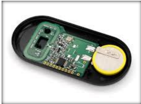
Plate 2.56: Shows an Active electronic tag opened to see the components (Source: www.learn.sparkfun.com )
