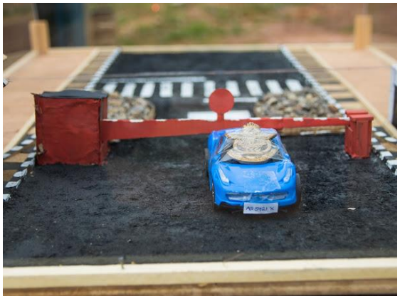
Plate 3.88: Shows the miniature vehicle as it passes through the barrier after successful authentication.
