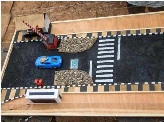
Plate 3.87: Shows linear actuator (barrier) opened up to allow the vehicle pass.
