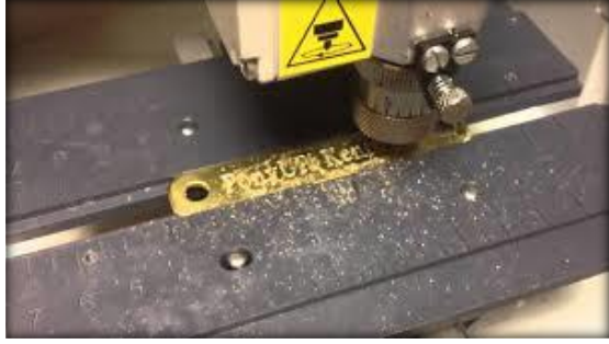
Plate 2.35: Shows an engraving machine being used to engrave a metal plate. (Source: www.signplus.com.au )
