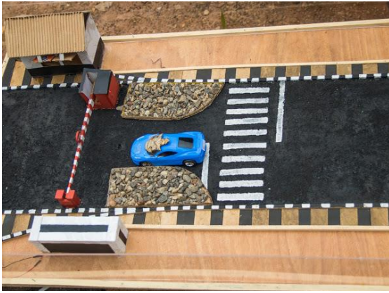
Plate 3.85: Shows the miniature vehicle Standing on the RFID reader to authenticate the identification and grant access number
