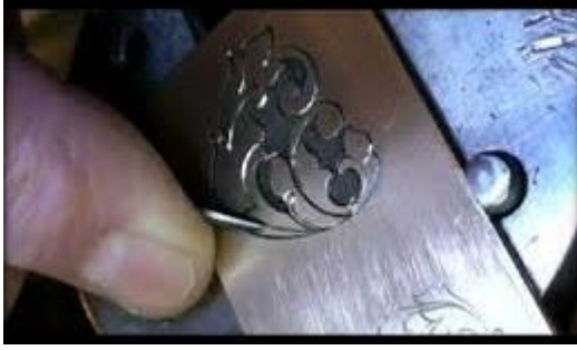
Plate 2.34: Shows a burin being used to engrave a metal plate (Source: www.embeddedtronics.com )
