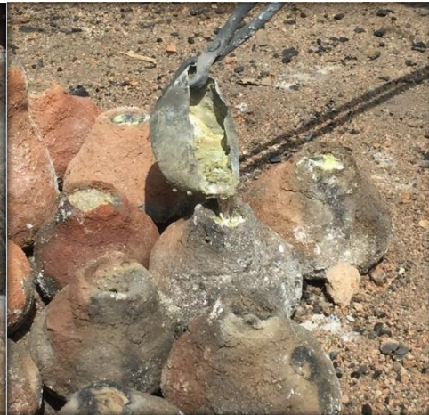
Plate 3.70: Shows pouring of molten metal in the dewaxed mould.
