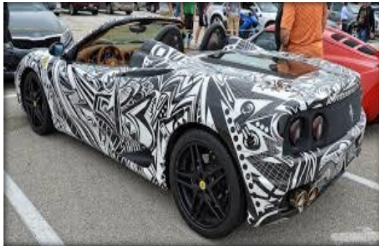
Plate 2.10: Shows a customised vinyl designed material wrapped around a vehicle (Source: www.ebay.com )
