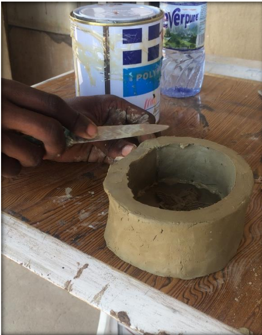
Plate 3.33: Shows building of wall around the model for the POP mould
