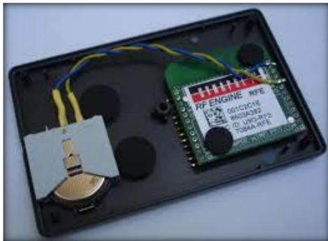
Plate 2.60: Shows an Active electronic tag Opened to see the components (Sources: www.promageurope.com )
