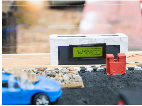
Plate 3.86: Shows the displayed screen displaying the name of the owner of the vehicle and the vehicle's registration number
