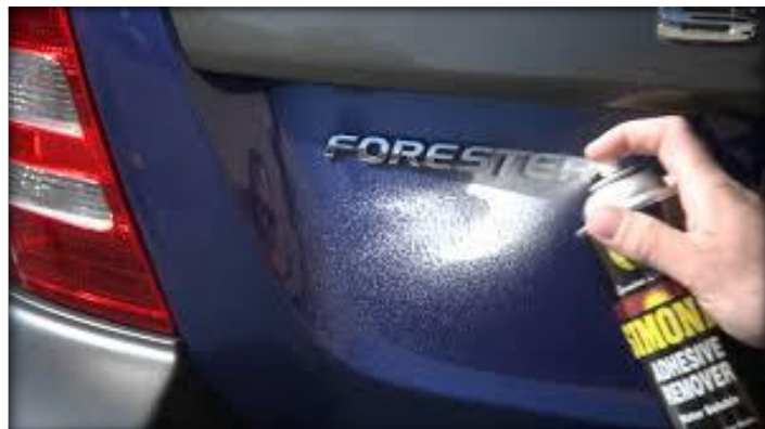
Plate 2.19: Shows a solvent-based adhesive remover being sprayed onto an adhered impression (Source: www.wikihow.com )
