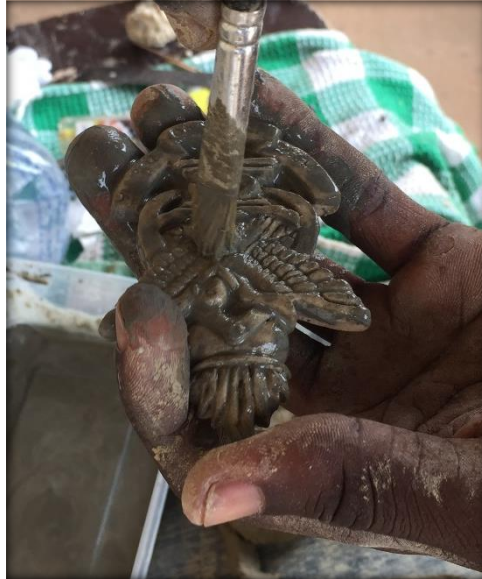
Plate 3.56: Shows applying of slurry cement on the model to pick all the intricate design.
