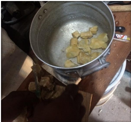
Plate 3.46: Shows bee wax being heated aluminium bowl with the aid of blow torch
