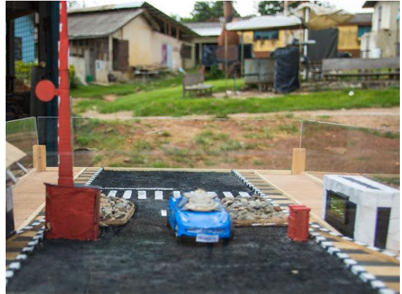
Plate 3.90: Shows the linear actuator raised up as the vehicle stands on the sensor area.
