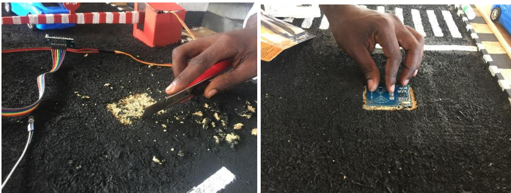
Plate 3.19: Shows cutting a space to fix the RFID reader. Plate 3.20: Shows fixing the RFID reader.
