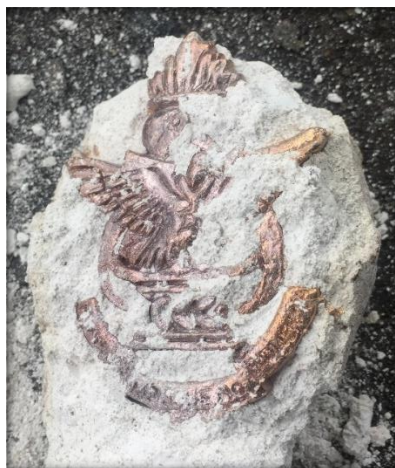
Plate 3.71: Shows the breaking of the mould. After breaking the mould to obtain the cast piece, the runners were cut off with hack saw.
