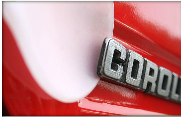
Plate 2.22: Shows a plastic putty knife tilted behind the impression for easy peeling.
