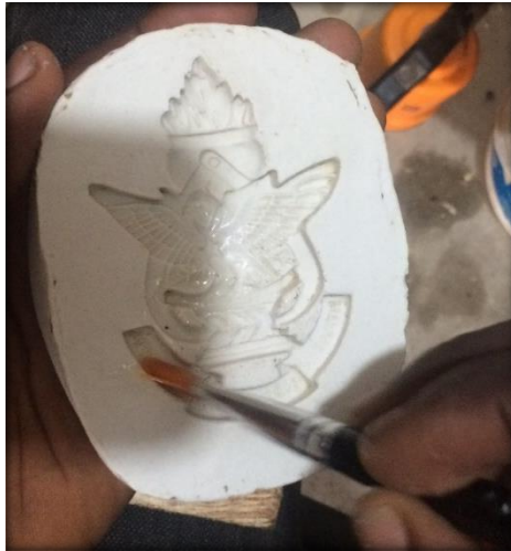
Plate 3.48: Shows cooking oil (frytol) being spread in the POP mould for wax picking.
