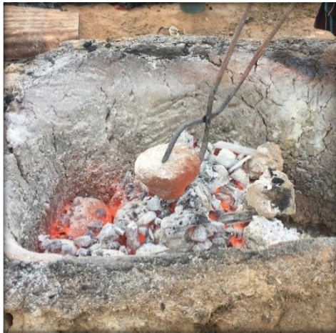
Plate 3.69: Shows removing of dewaxed mould.
