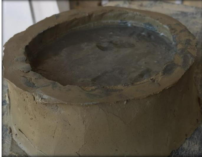
Plate 3.58: Shows the cavity filled with the slurry cement.
