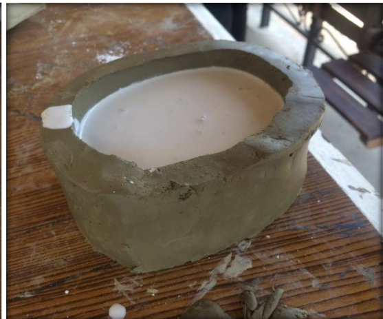
Plate 3.38: Shows the slurry POP being poured into the mould to settle.
