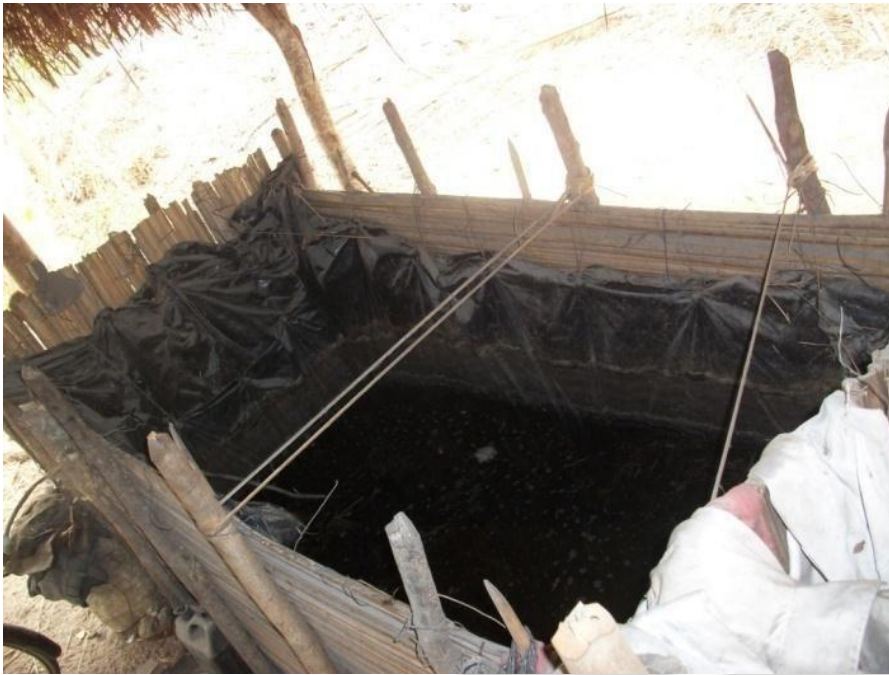
Fig. 6: A reservoir (local condenser) which stores water for condensing the alcohol vapour during the distillation of “akpeteshie” (the local gin) at Kakadedzi
