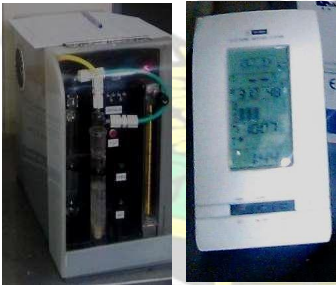
Figure 3.2: Picture of System Service Innovation Incorporation air sampler model 1000i and 433 MHz Electronic Weather station
