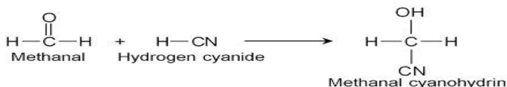
Figure 2.2: Reaction of formaldehyde with hydrogen cyanide
