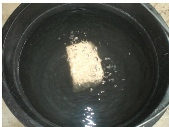
**Plate 3.58: Water filling air pockets in the fired brick**
