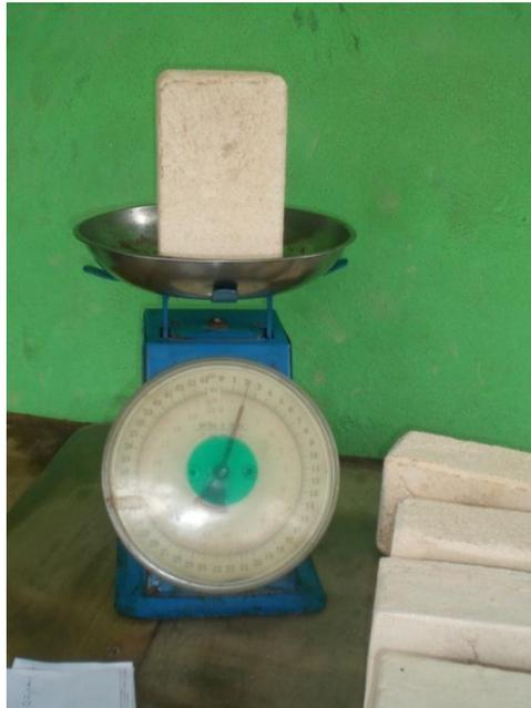
**Plate 3.56: Researcher weighing the fired bricks to check the reduction in masses**
