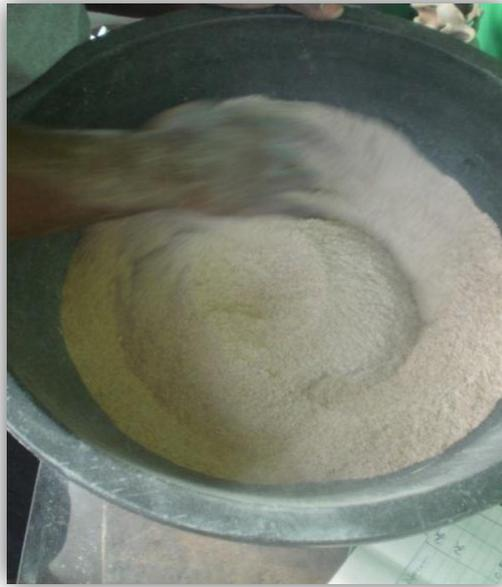
**Plate 3.45: Researcher mixing Kenyase Abrem and Tapa clay together with sawdust, thoroughly with the hand**
