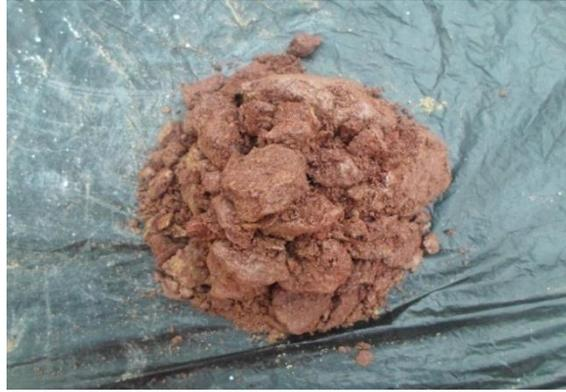
**Plate 2.1: Abonko clay in the dry state fetched from the parent rock**
