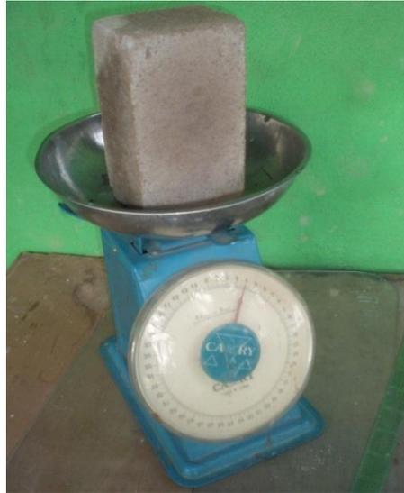
**Plate 3.54: Researching weighing the mass of the dried bricks**
