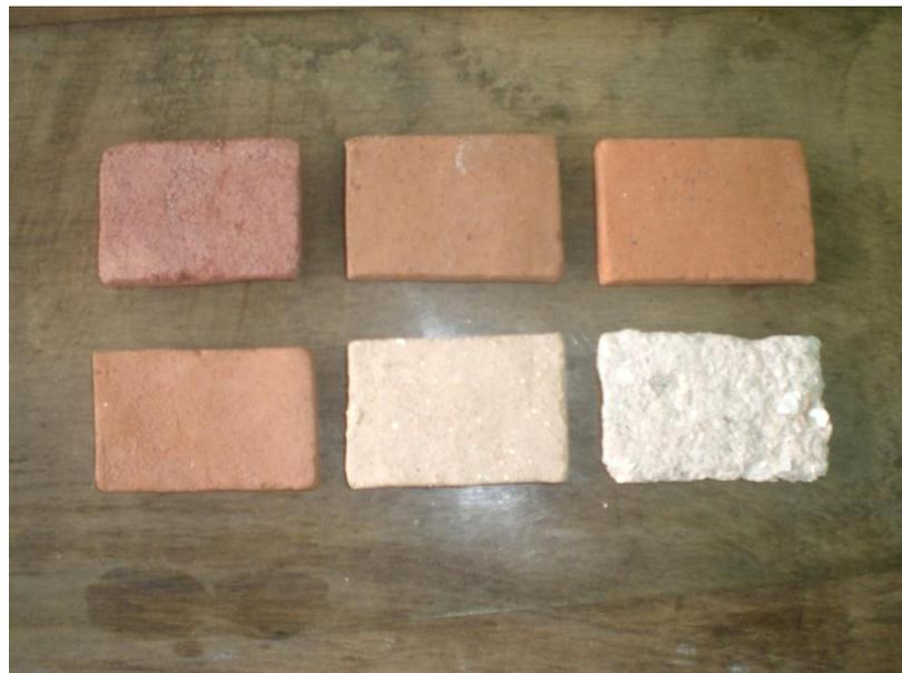
**Plate 3.39: Colour of the tested clay samples fired when fired to 1100°C (2012°F)**
