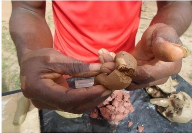
**Plate 3.22: Researcher checking the plasticity of Abonko Clay fetched two (2) meters around parent rock**
