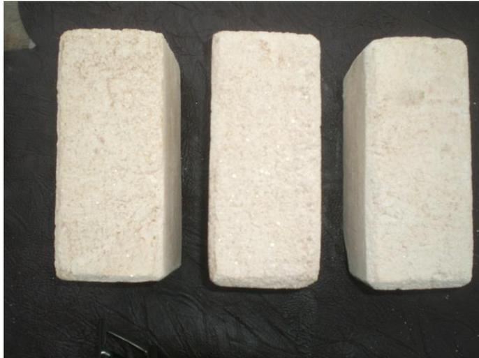
**Plate 4.3: Colour and surface texture brick made from experiment 1, 2 and 3**
