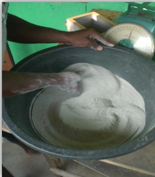
**Plate 3.44: Researcher mixing the two clays homogeneously**
