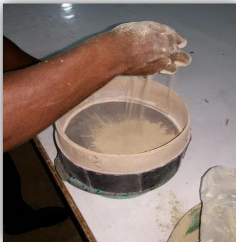
**Plate 3.42: Researcher sieving the pulverized clays into finer particles with a 90mesh sieve**
