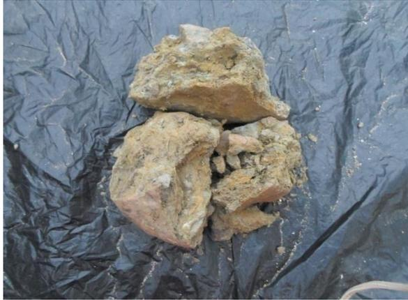
**Plate 2.4: Adankwame clay sample in the dry state**
