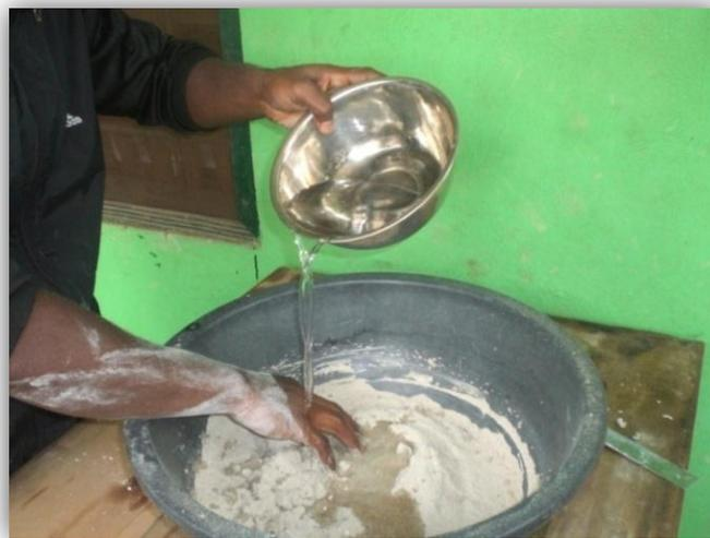
**Plate 3.46: Researcher adding water to the mixture of the two clays and sawdust.**
