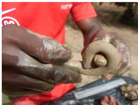
**Plate 3.24: The researcher checking the plasticity of Adankwame clay**
