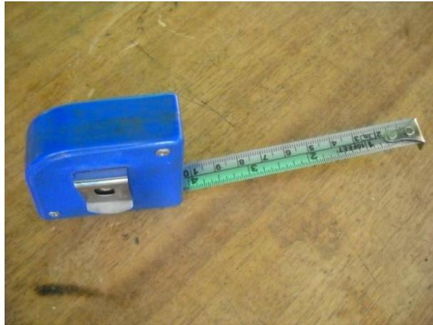
**Plate 3.3: Carpenter's tape measure**
