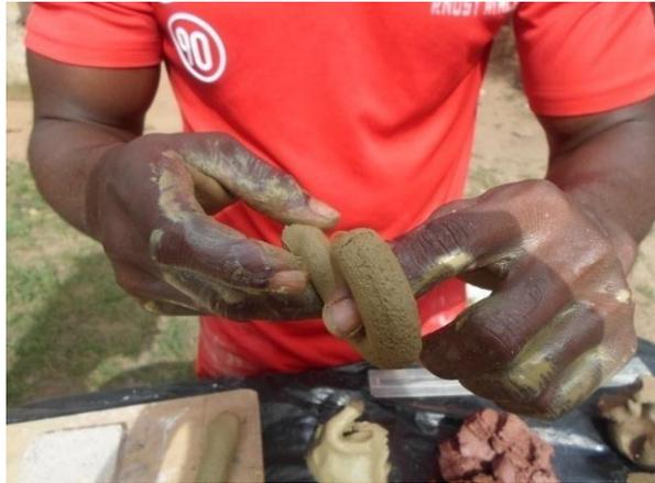
**Plate 3.23: The researcher checking the plasticity of Abonko Clay from secondary source**
