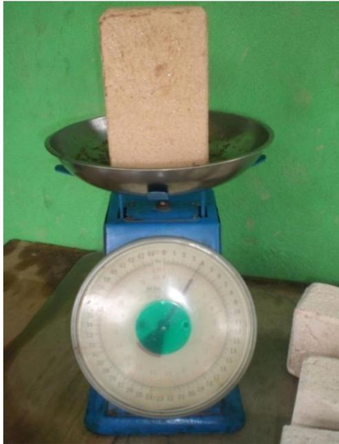
**Plate 3.59: Researcher weighing the mass of bricks right after it has been completely soaked in water**
