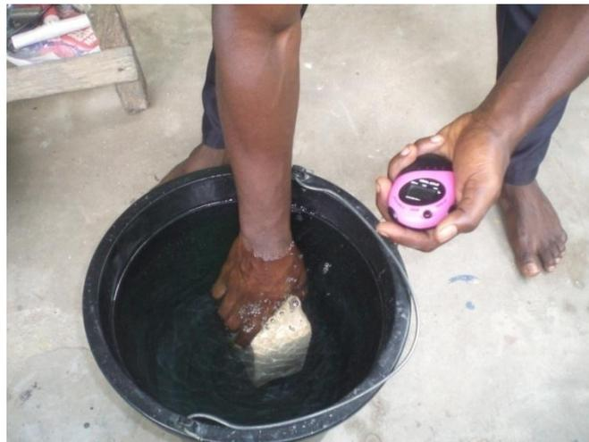
**Plate 3.57: Researcher putting fired brick in boiled water to check open porosity and water absorption**
