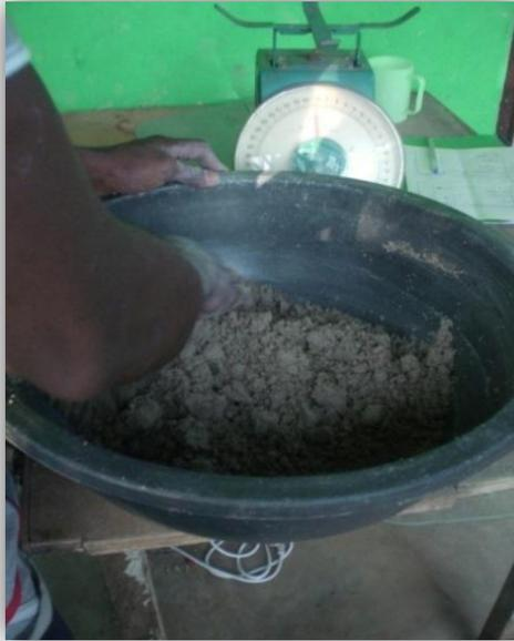
**Plate 3.47: Researcher mixing composition into a uniform consistency after adding water**
