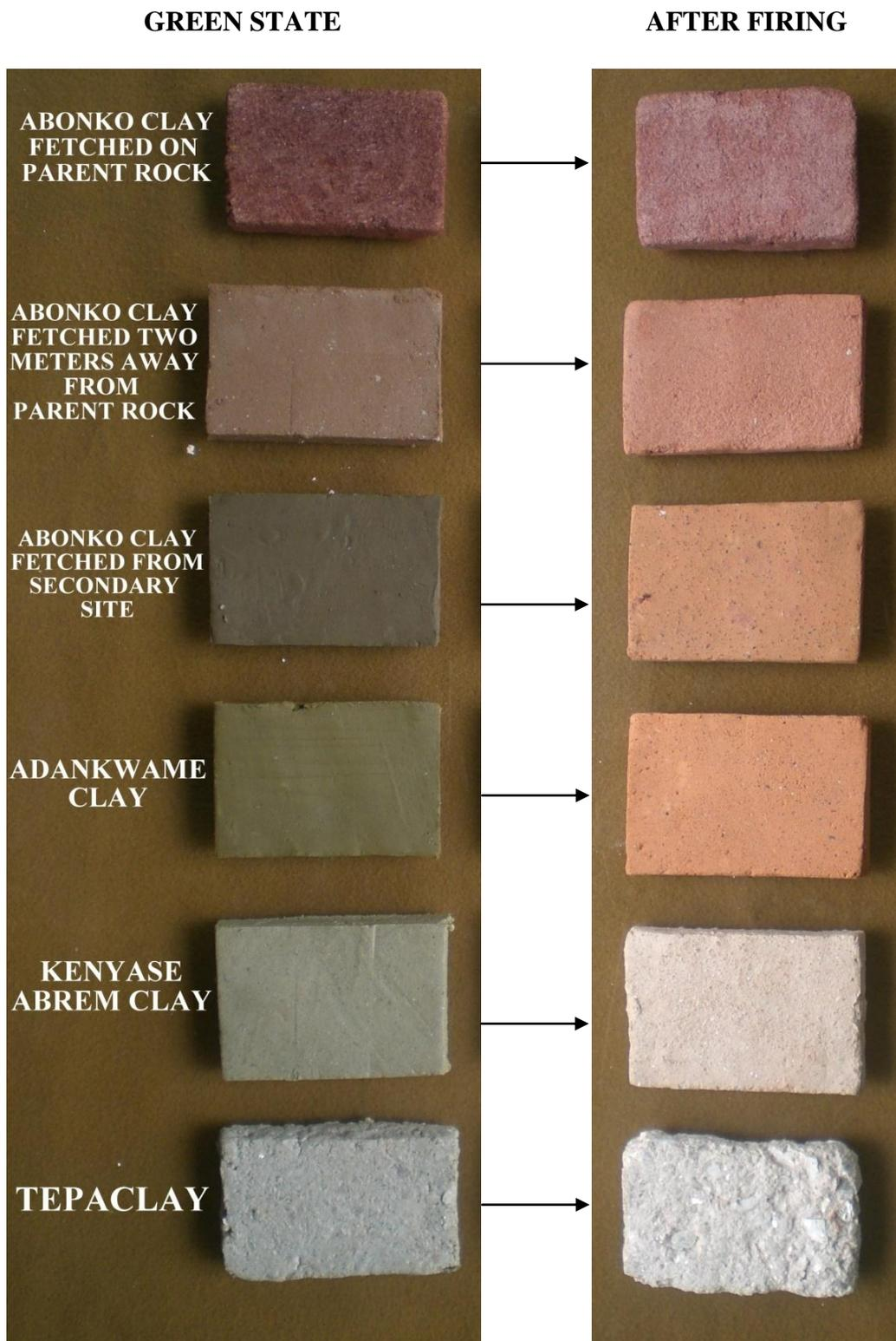
Plate 4.2: Colour transformation in the six (6) clays after they were fired to 1100
