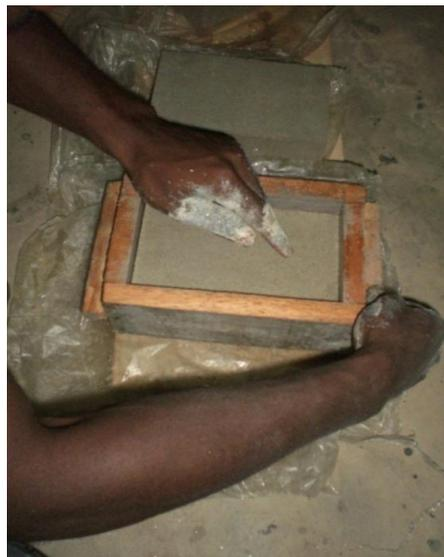
**Plate 3.51: Researcher pushing the molded brick out of the mould**
