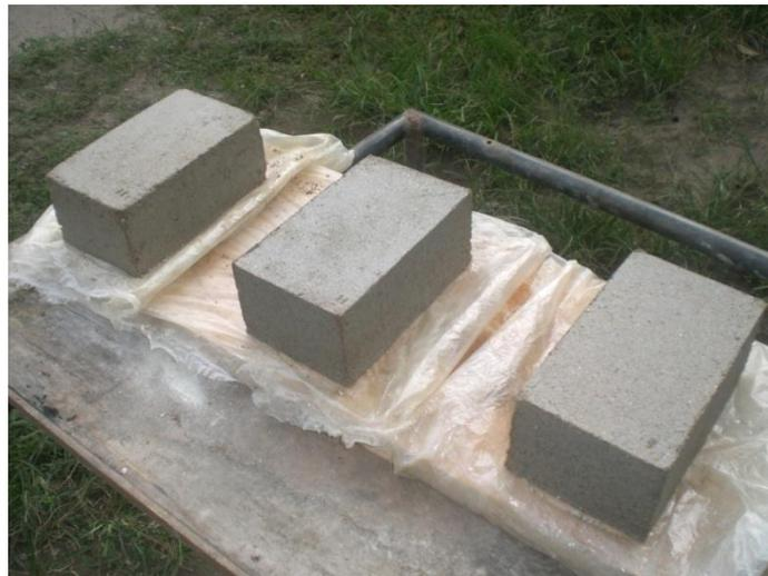
**Plate 3.53: Drying of the bricks.**
