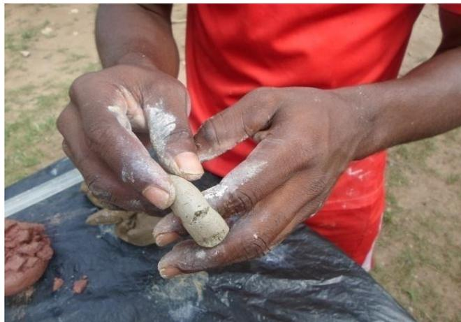
**Plate 3.25: The researcher checking the plasticity of Kenyase Abrem Clay**
