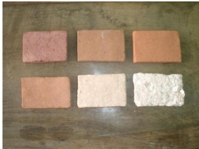
**Plate 4.1: Fired clay samples from each of the six (6) clays.**
