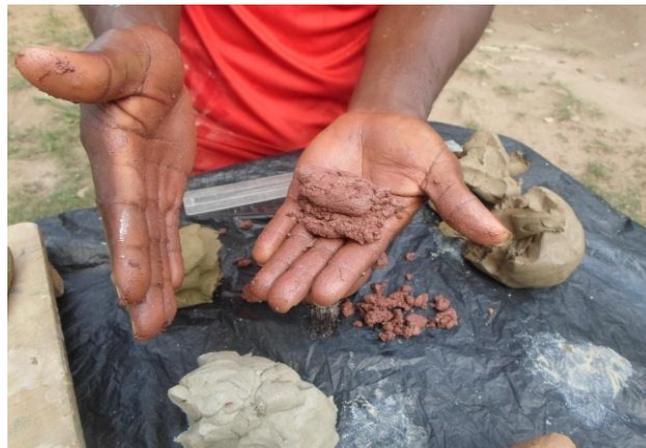
**Plate 3.21: The researcher checking the plasticity of Abonko Clay fetched from parent rock**
