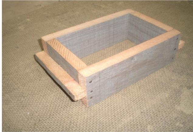
**Plate 3.5: Wooden brick mould**
