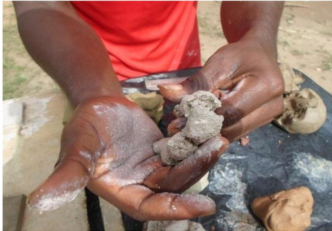
**Plate 3.26: The researcher checking the plasticity of Tewa clay**
