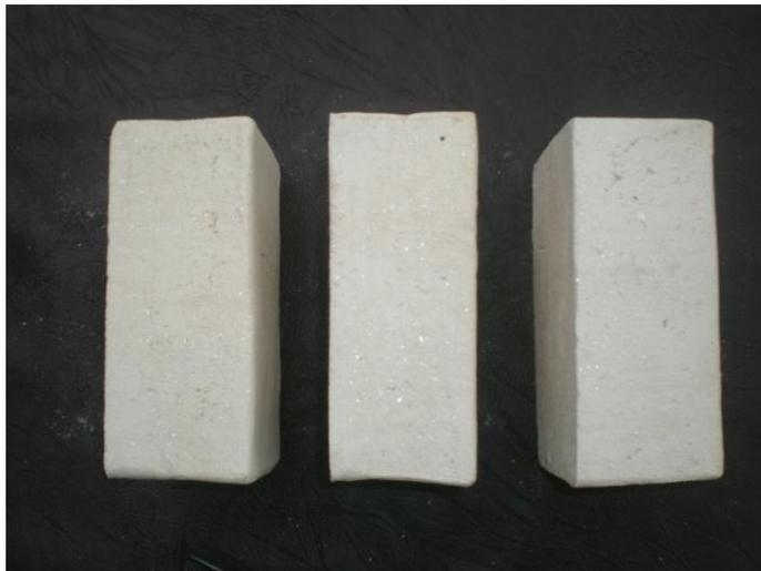
**Plate 3.4: Colour and surface texture brick made from experiment 4, 5 and 6**
