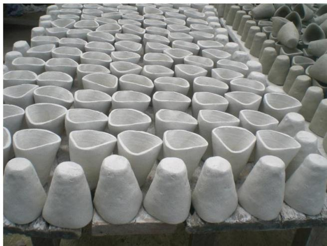
**Plate 3.18: Crucibles made from Kenyase Abrem Clay because of its refractoriness**
