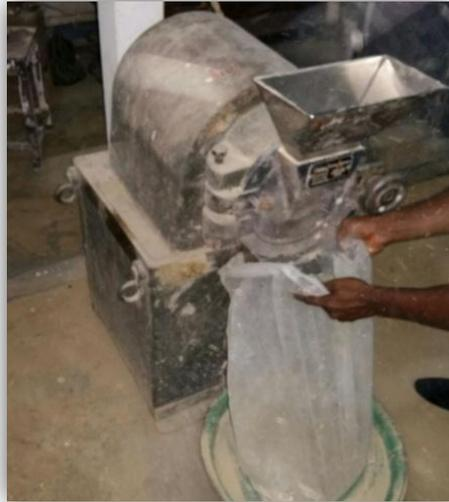
**Plate 3.41: Researcher pulverizing the clay in a pulverizing machine into a fine state**
