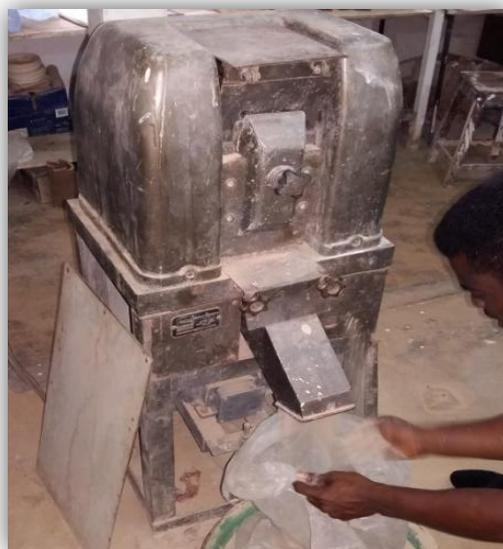
**Plate 3.40: Researcher crushing clay into smaller particles in a jaw crusher**
