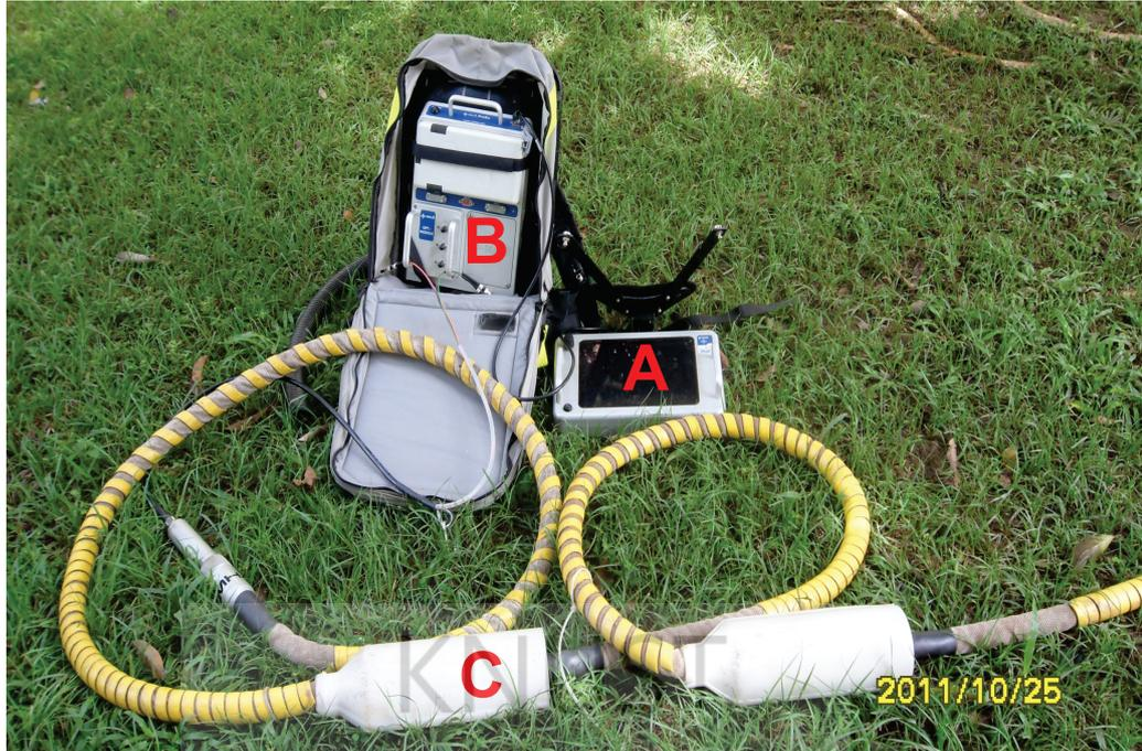
Figure 4.2: MALA GPR equipment used for the survey: A is XV monitor, B is Control unit, C is the RTA
