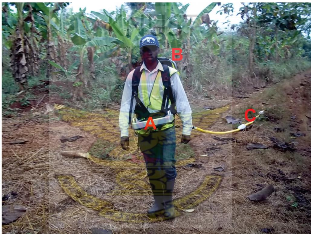
Figure 4.3: GPR data collection in a continuous mode operation: A is the XV Monitor, B is the control unit and, C is the 100 MHz RTA antenna
