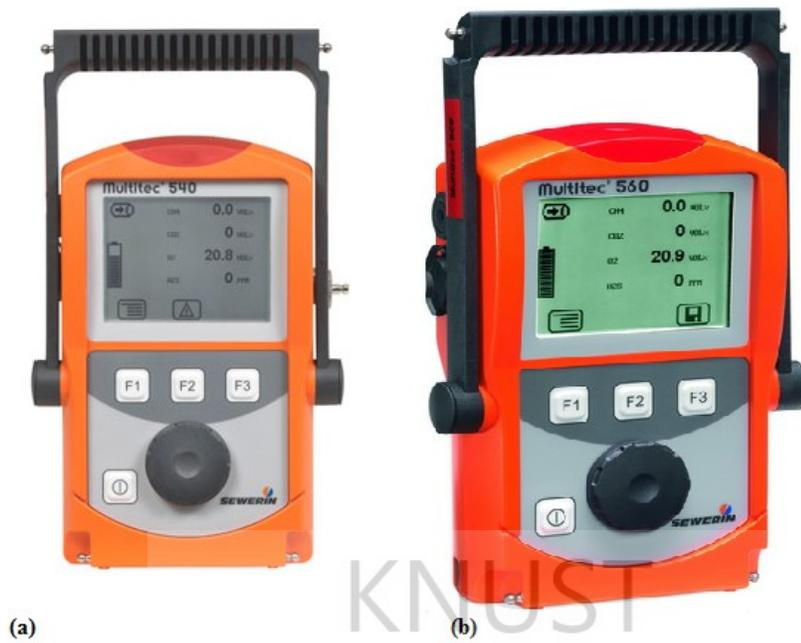
**Figure 2.23: Portable Electronic Biogas Analyzer: Multitec 540 and Multitec 560 manufactured by Sewerin Technologies (Adapted from [www.sewerin.com](http://www.sewerin.com))**
