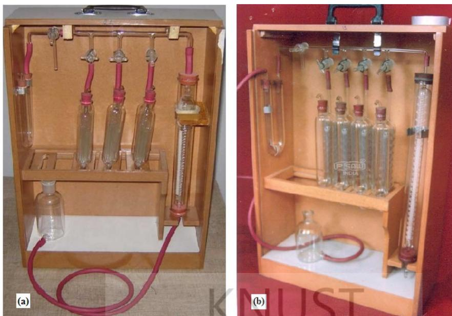
**Figure 2.22: The Orsat Apparatus (a) with three bulbs in series (b) with four bulbs in series (both pictures were adopted from Google)**
