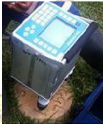
Figure 4.3: Scintrex Autograv CG-5 gravimeter used for the survey
