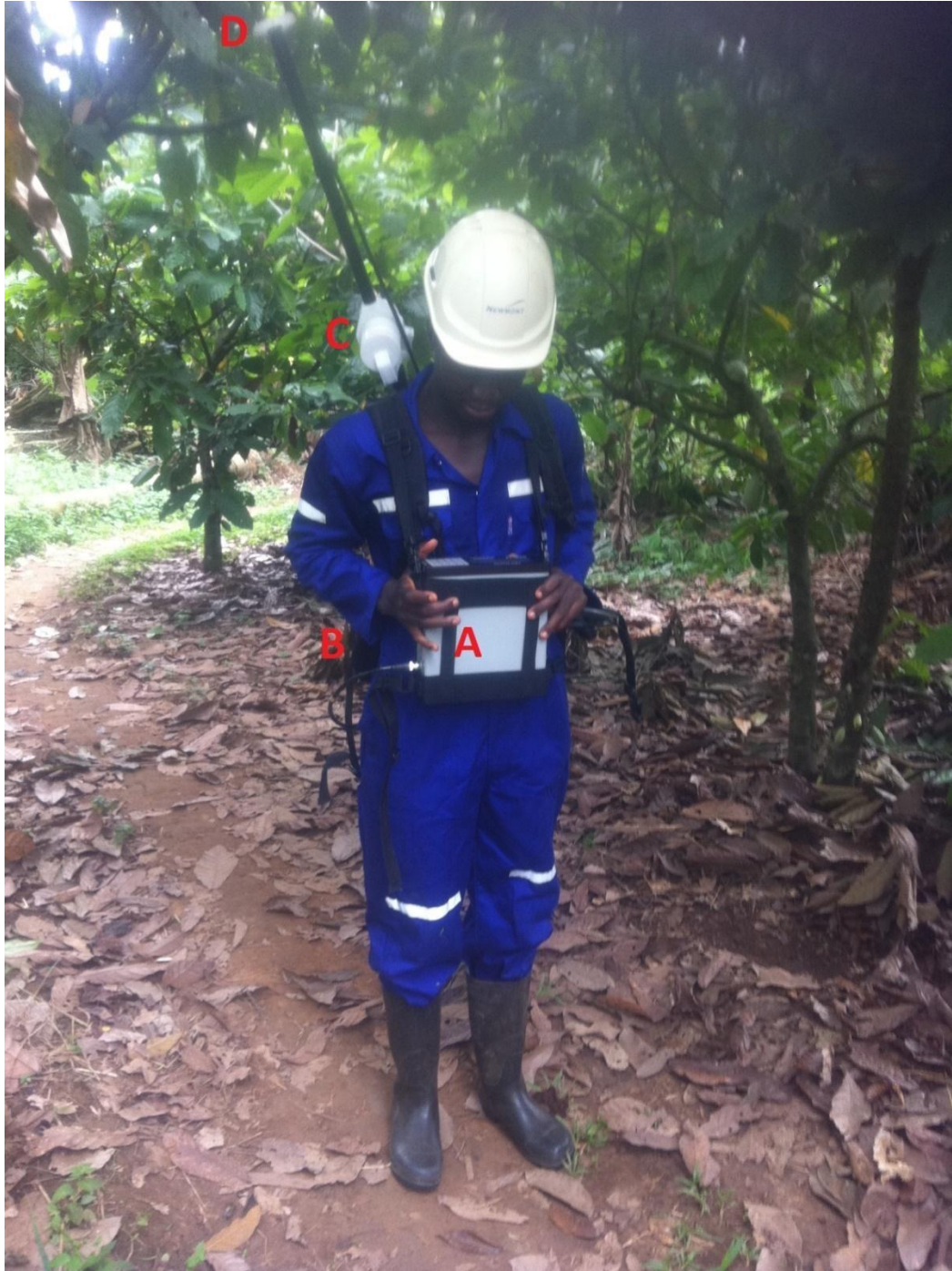
Figure 4.2: Magnetic survey in progress with Overhauser magnetometer. A- Control unit, processor and monitor, B- battery backpack, C-Sensor, D-GPS antenna (Photo: Seth, 2015)
